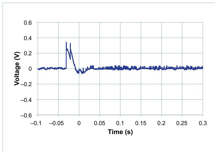
**Figure 12** — Transient response of the VS1 (+12V) output with a load step of 100% (40A) to 0%; AC coupled
