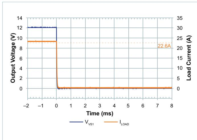
**Figure 18** — Discharge time of the VS1 (+12V) output
