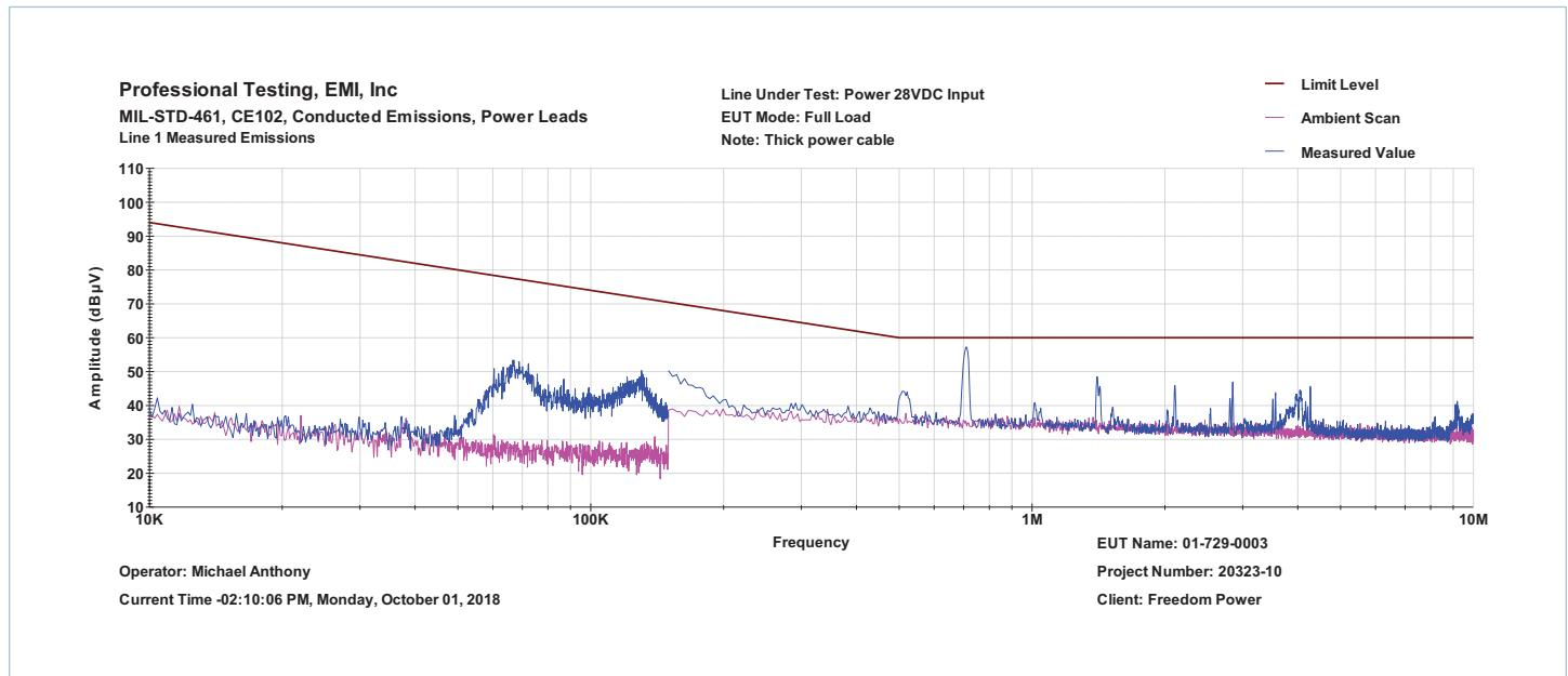
**Figure 29** — Conducted emissions of  $28V_{DC}$  input at full load
