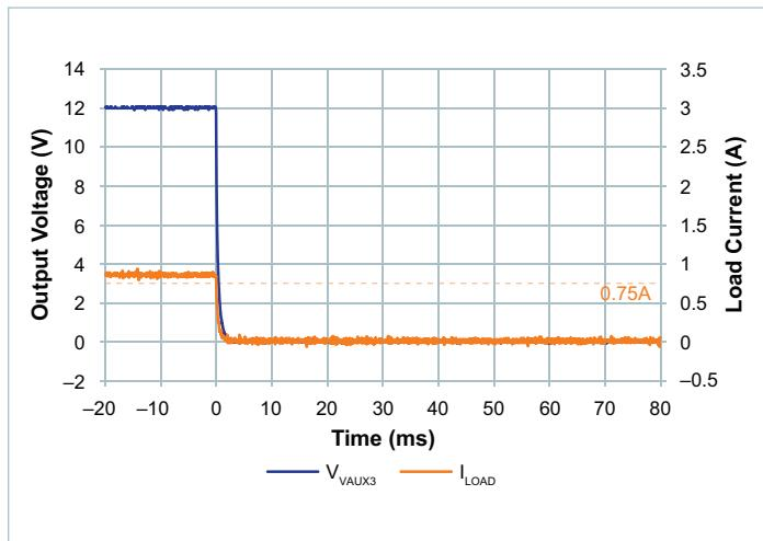
**Figure 24** — Discharge time of the VAUX1 (-12V) output
