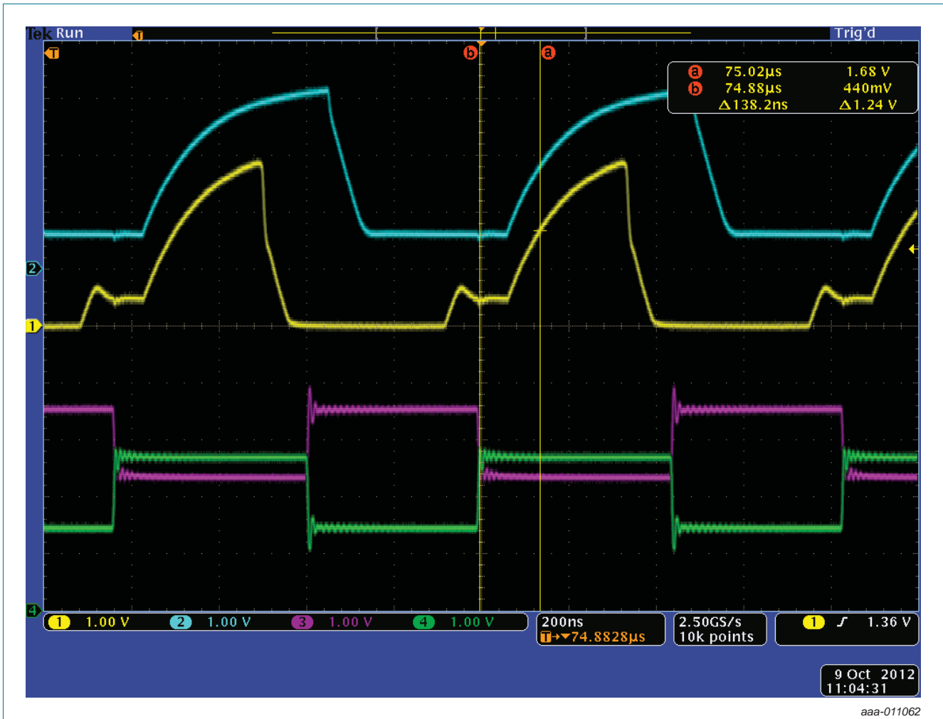
Fig 9. Differential bus waveform
