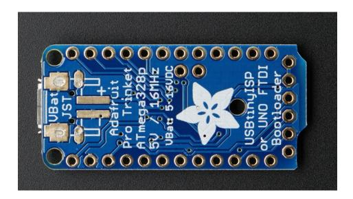
On the bottom there's a spot for a 2-pin JST-PH connector (http://adafru.it/1769). this is optional and can be soldered on by hand. It will let you use a lipoly or AAA battery pack (http://adafru.it/727) or a JST cable (https://adafru.it/drM) for other power input. It's connected to the GND and VBAT pins
