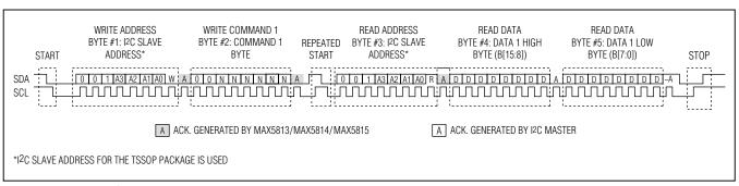
Figure 6. Standard I<sup>2</sup>C Register Read Sequence
