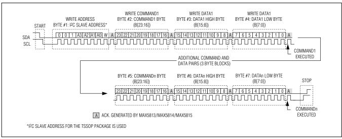
Figure 5. Multiple Register Write Sequence (Standard I<sup>2</sup>C Protocol)
