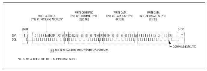
Figure 4. I<sup>2</sup>C Single Register Write Sequence
