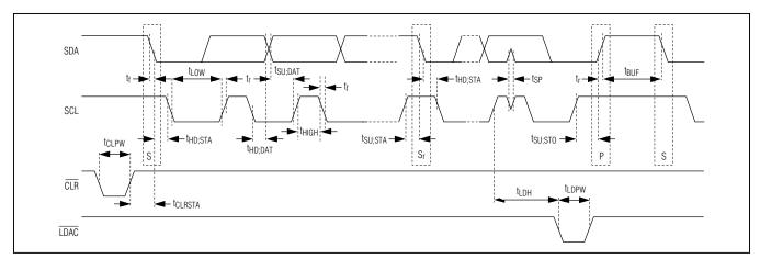
Figure 1. I<sup>2</sup>C Serial Interface Timing Diagram
