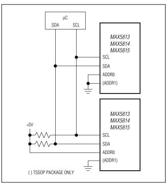
Figure 8. Typical I<sup>2</sup>C Application Circuit
