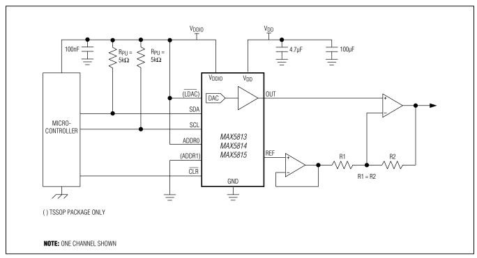
Figure 9. Bipolar Operating Circuit
