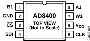
Figure 6. AD8400 Pin Configuration
