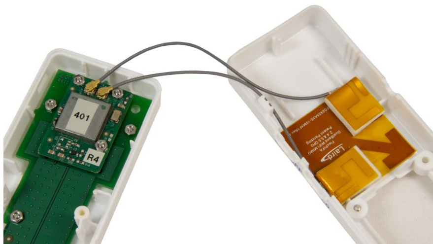
Figure 2: Typical placement of FlexPIFA MIMO within a plastic electronic package
