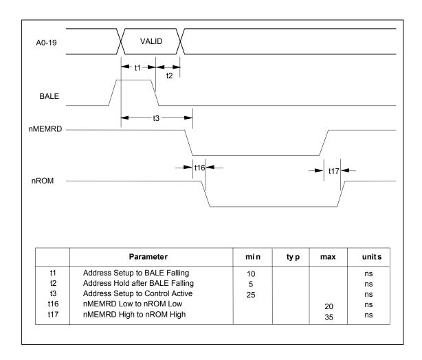
Figure 12.9 - External ROM Read Access Using Bale
