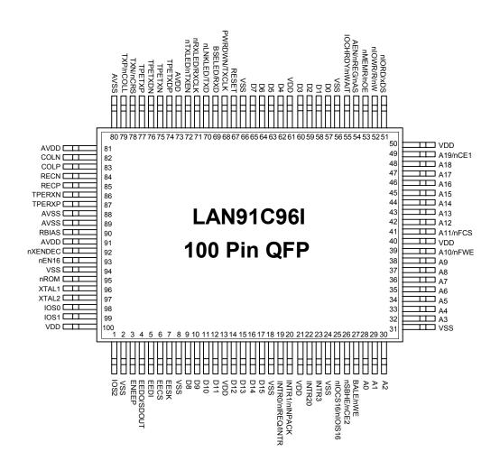
Figure 3.1 - Pin Configuration of LAN91C96I QFP
