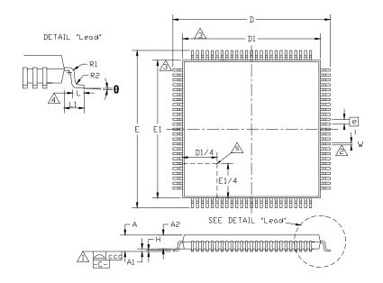
Figure 13.2 - 100 Pin TQFP Package Outline
