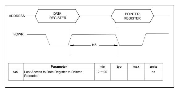
Figure 12.21 – Memory Write Timing
