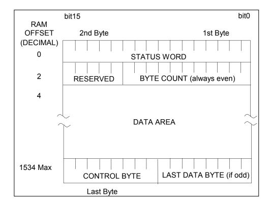
Figure 6.1 - Data Packet Format
