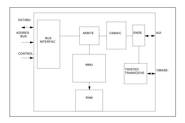
Figure 4.1 - LAN91C96l Internal Block Diagram
