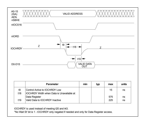
Figure 12.4 – Data Register Special Read Access
