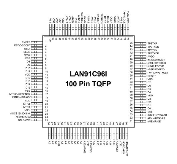
Figure 3.2 – Pin Configuration of LAN91C96I TQFP
