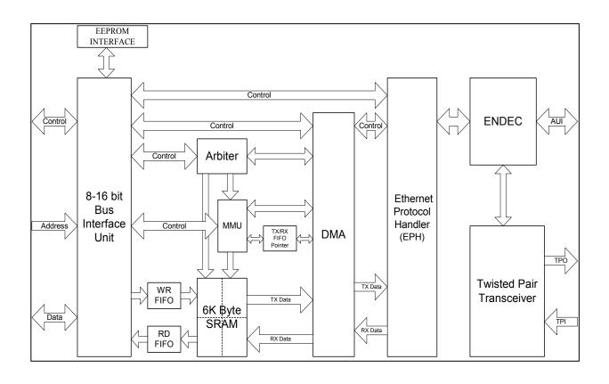
Figure 5.4 - LAN91C96i Internal Block Diagram with Data Path
