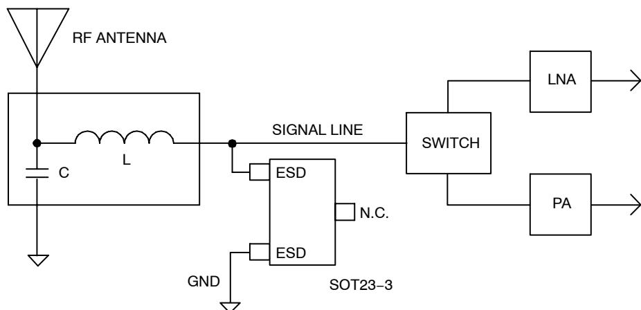
**Figure 7. Typical Application – RF Switch and Amplifier Protection,
