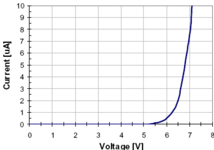
**Figure 3. CM1214A VI Characteristics,
