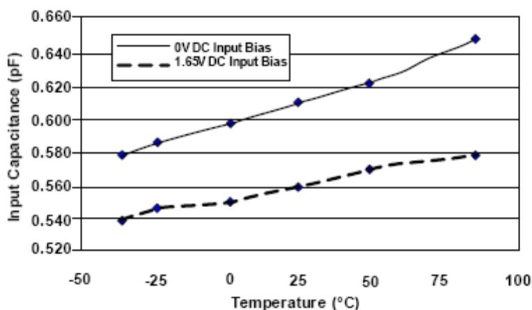
**Figure 4. CM1214A Capacitance vs. Temperature**
