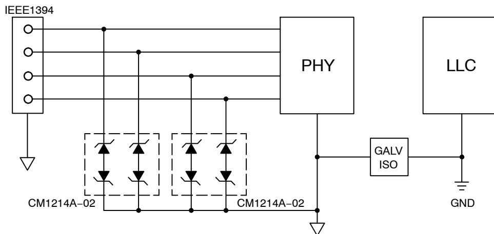
Keep the ESD devices on the PHY side of the galvanic isolation and inside the V<sub>CC</sub> domain of the PHY controller
