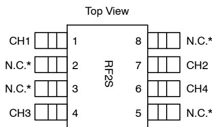
\* All N.C. pins must be left floating (i.e., not connected to the PCB). See applications section for more information.
