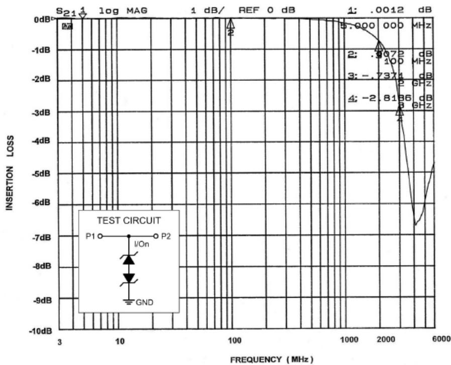
Figure 6. Insertion Loss vs. Frequency (2.5 V DC Bias)
