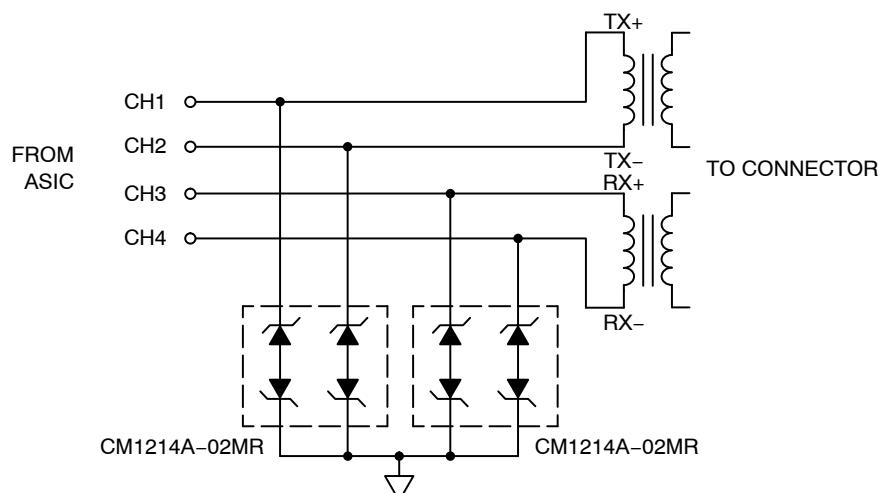
**Figure 8. Typical Application – Ethernet Protection,
