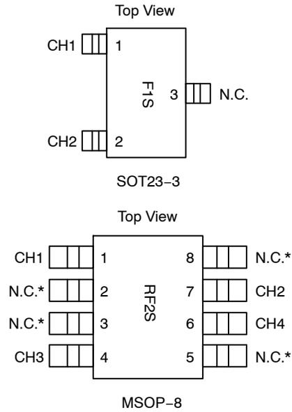
\* All N.C. pins must be left floating (i.e., not connected to the PCB). See applications section for more information.
