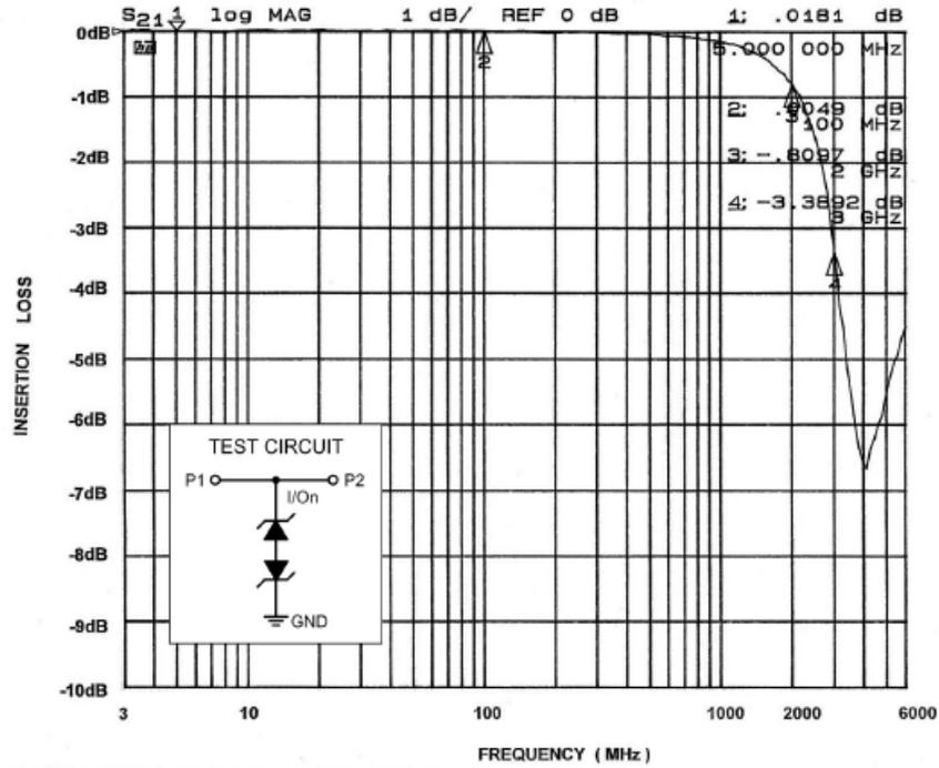
Figure 5. Insertion Loss vs. Frequency (0 V DC Bias)
