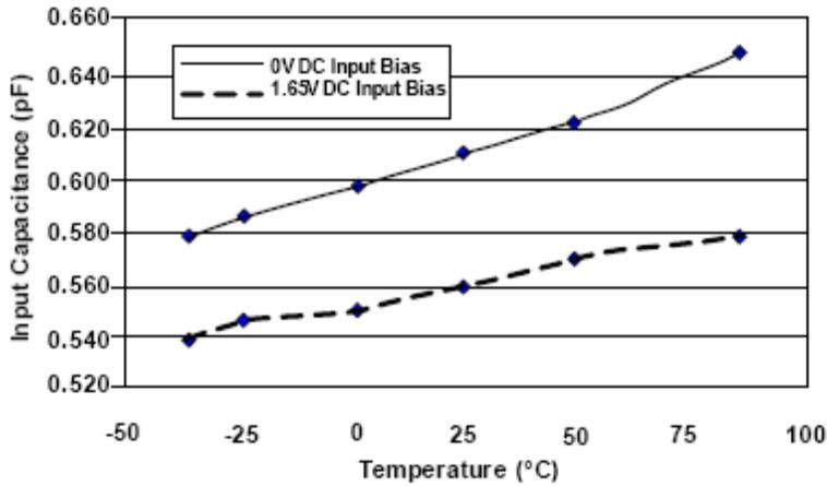
Figure 4. CM1214A Capacitance vs. Temperature
