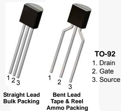
Figure 1. J175 / J176 Device Package
