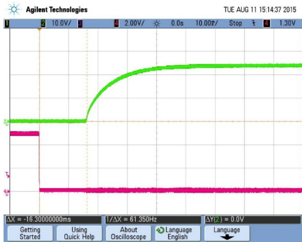
Turn-on transient at zero load current (10 mS/div, Top Trace: Vout, 10V/div; Bottom Trace: ON/OFF, 2V/div)
