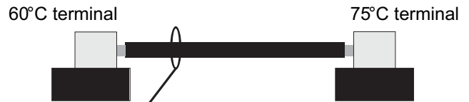
Conductor size and insulation rating?
