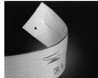
Pre-manufactured Slit-and-Twist Cable (R-CAM 4 only)
