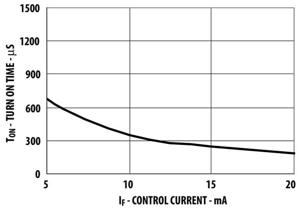
Figure 12. Typical Turn On Time vs Input Current
