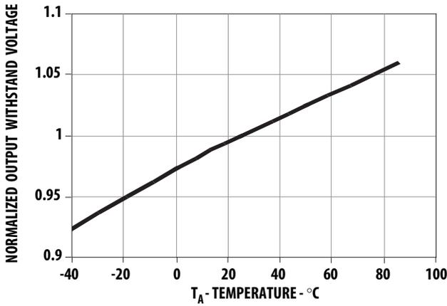
Figure 3. Normalized Typical Output Withstand Voltage vs Temperature
