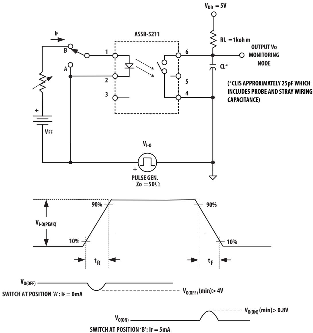
Figure 18 . Test Circuit for Input-Output Transient Immunity
