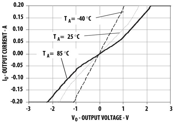
Figure 9. Typical Output Current vs Output Voltage
