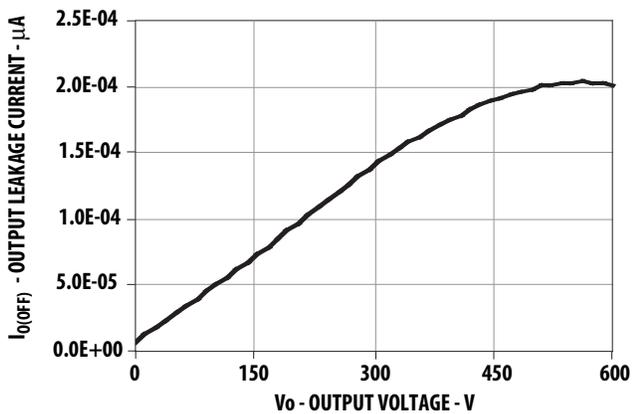
Figure 5. Typical Output Leakage Current vs Output Voltage
