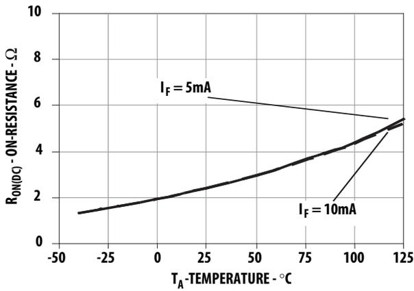
Figure 11. Typical On Resistance (DC Connection) vs Temperature
