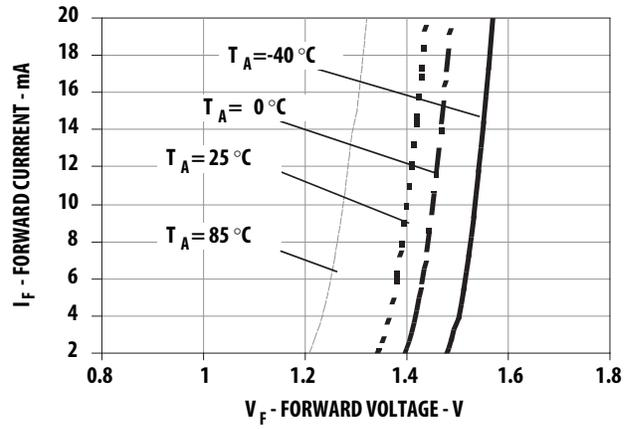
Figure 8. Typical Forward Current vs Forward Voltage
