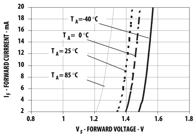
Figure 8. Typical Forward Current vs Forward Voltage
