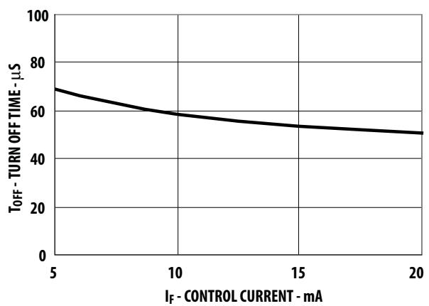
Figure 14. Typical Turn Off Time vs Input Current
