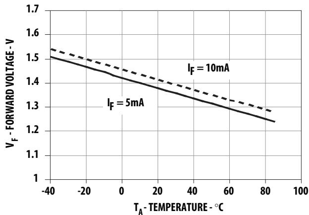
Figure 7. Typical Forward Voltage vs Ambient Temperature
