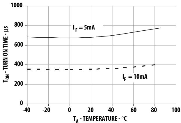
Figure 13. Typical Turn On Time vs Temperature
