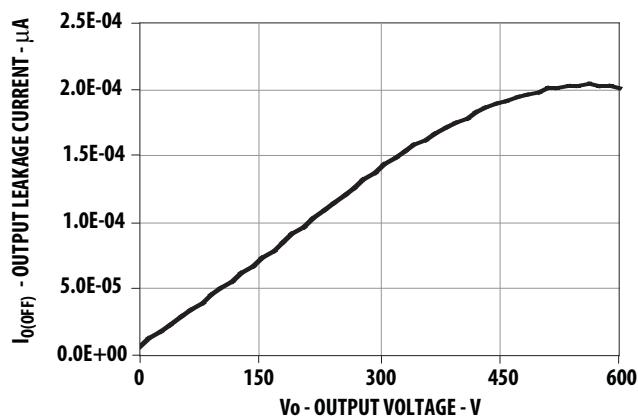
Figure 5. Typical Output Leakage Current vs Output Voltage
