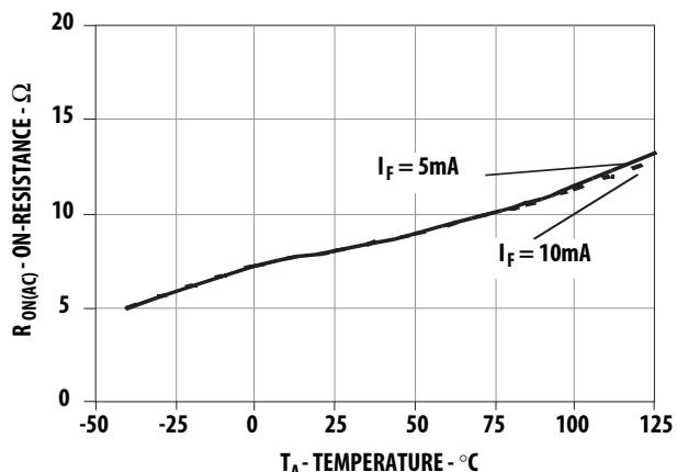
Figure 10. Typical On Resistance (AC/DC Connection) vs Temperature
