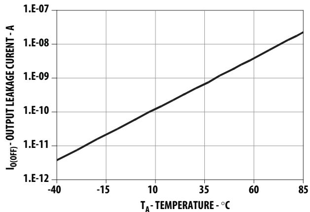
Figure 4. Typical Output Leakage Current vs Ambient Temperature
