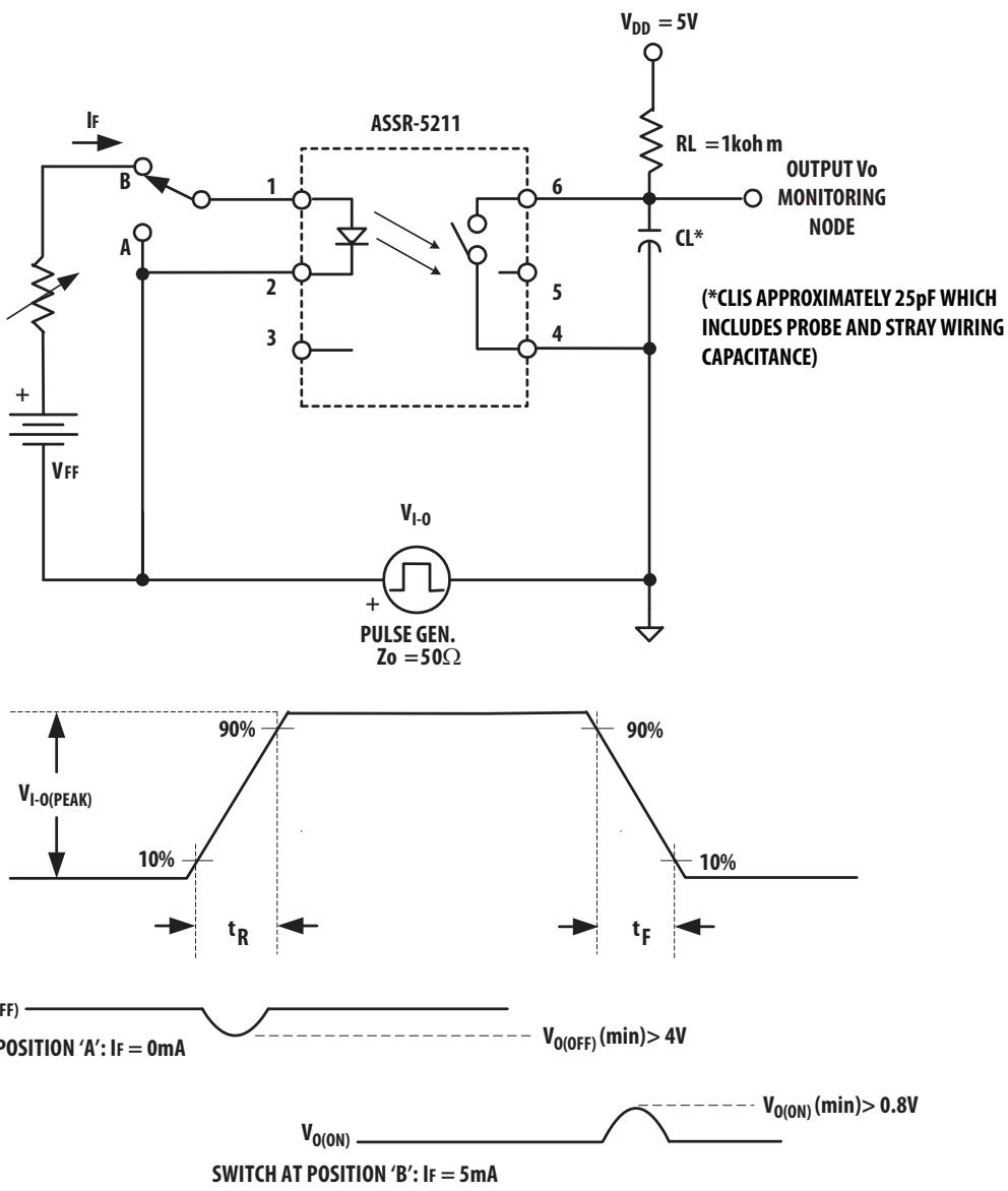
Figure 18 . Test Circuit for Input-Output Transient Immunity
