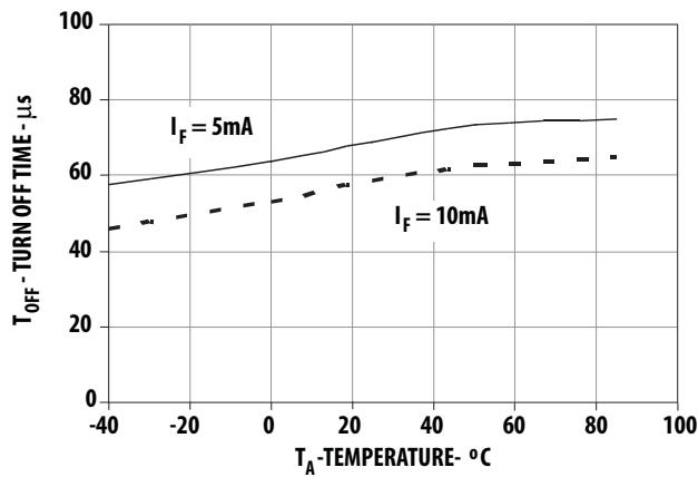
Figure 15. Typical Turn Off Time vs Temperature
