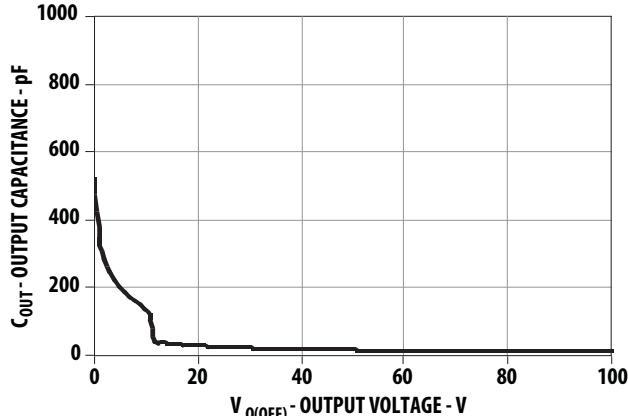
Figure 6. Typical Output Off-State Capacitance vs Output Voltage
