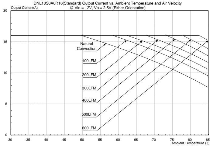
**Figure 33:** DNL10S0A0R16(Standard) Output current vs.
