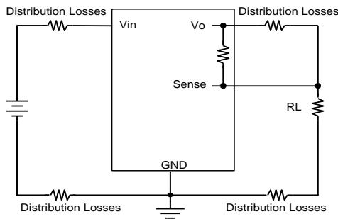
**Figure 23:** Effective circuit configuration for remote sense operation
