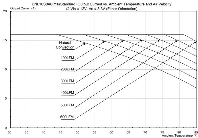
**Figure 32:** DNL10S0A0R16(Standard) Output current vs.
