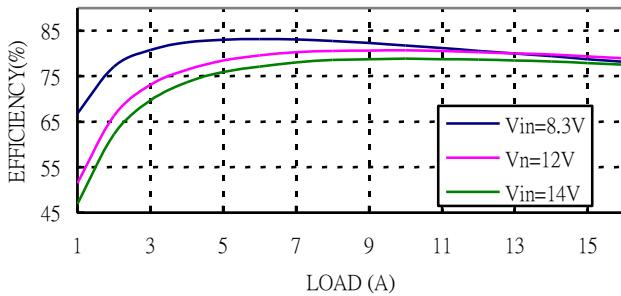
**Figure 1:** Converter efficiency vs. output current
