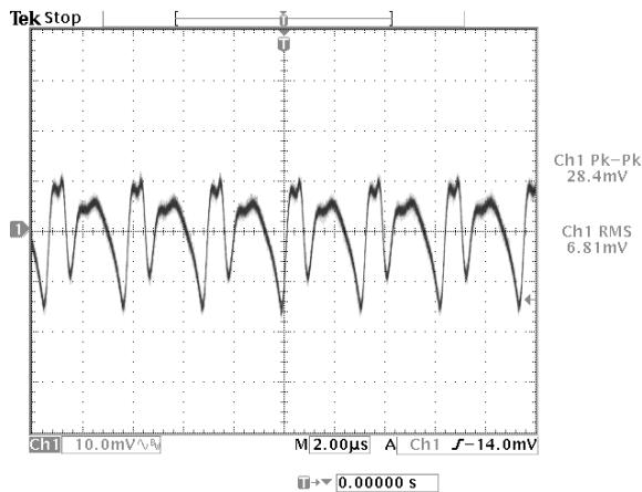
**Figure 8:** Output ripple & noise at 12Vin, 2.5V/16A out
