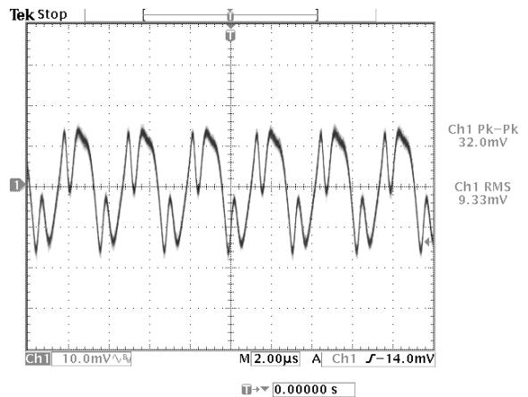
**Figure 9:** Output ripple & noise at 12Vin, 5.0V/16A out
