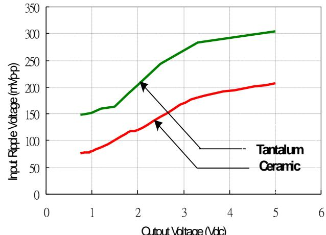
**Figure 20:** Input ripple voltage for various output models,
