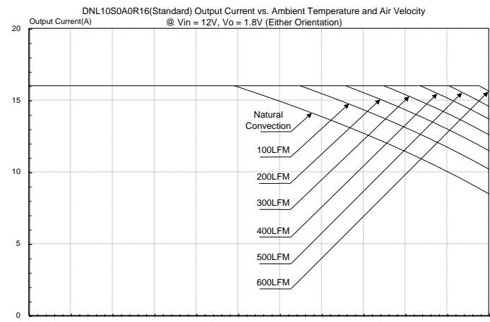
**Figure 34:** DNL10S0A0R16(Standard) Output current vs.
