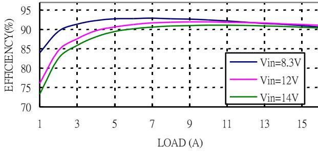
**Figure 5:** Converter efficiency vs. output current
