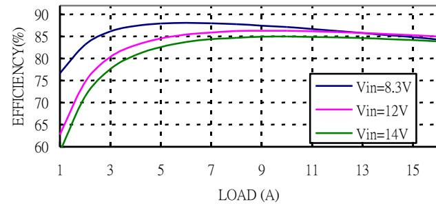
**Figure 2:** Converter efficiency vs. output current
