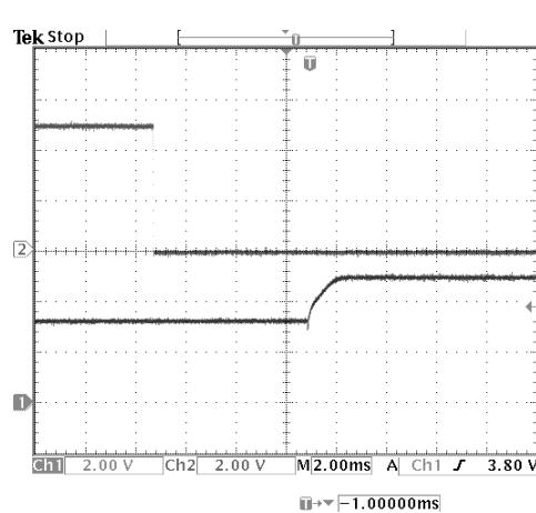
**Figure 16:** Turn on with Prebias 12Vin, 5V/0A out,  $V_{bias} = 3.3Vdc$
