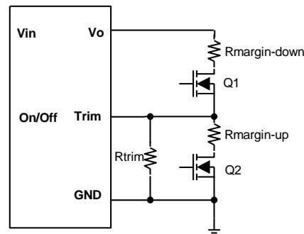
**Figure 26:** Circuit configuration for output voltage margining
