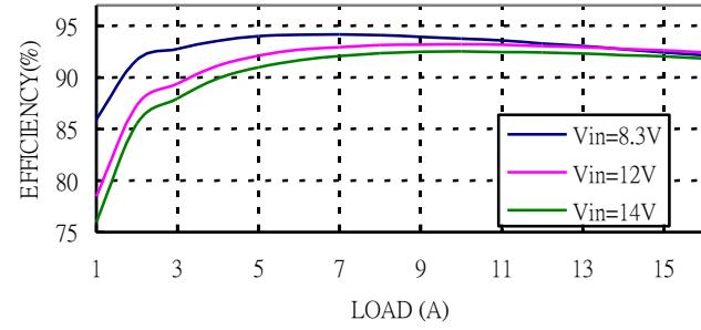
**Figure 6:** Converter efficiency vs. output current
