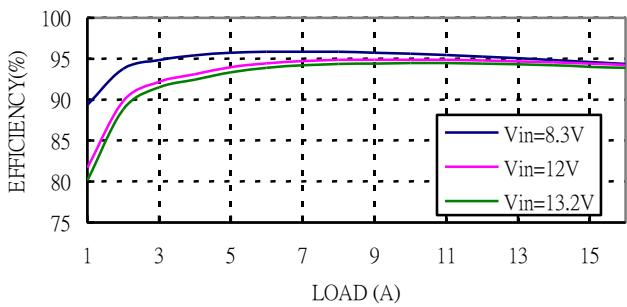
**Figure 7:** Converter efficiency vs. output current
