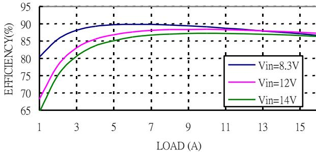
**Figure 3:** Converter efficiency vs. output current
