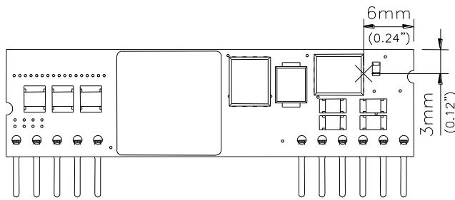
**Figure 31:** Temperature measurement location
