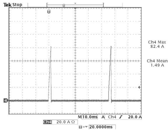
**Figure 15:** Output short circuit current 12Vin, 0.75Vout (10A/div)
