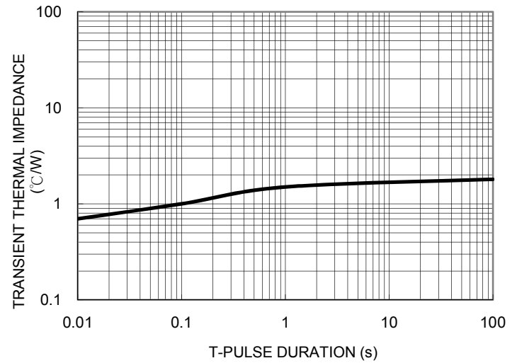
FIG. 8 TYPICAL TRANSIENT THERMAL IMPEDANCE PER LEG
