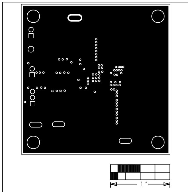
Figure 4. MAXM17543 EV Kit PCB Layout—PGND Layer 2
