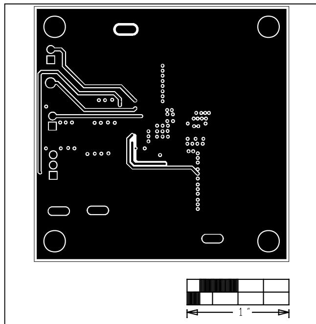
Figure 5. MAXM17543 EV Kit PCB Layout—PGND Layer 3
