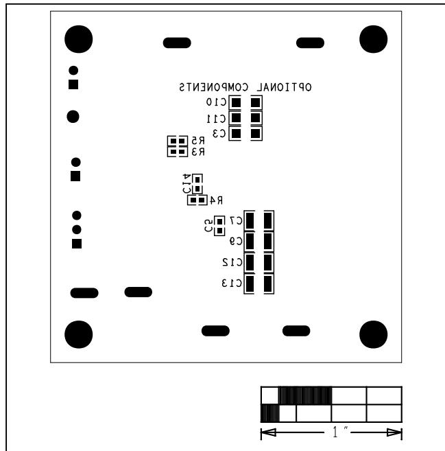
Figure 1. MAXM17543 EV Kit Component Placement Guide—
