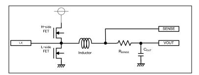
Figure A Detection with Sense Resistance
