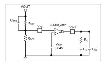
**Connection Example for External Phase Compensation Circuit**
