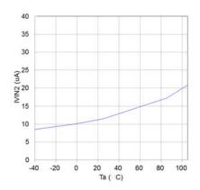
Current consumption (PWM)  $(V_{IN} = 12 V)$
