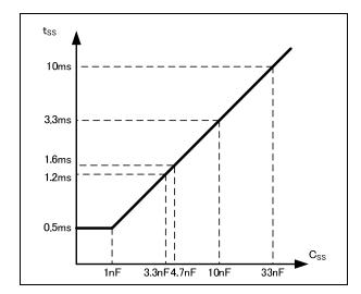
$C_{SS} [nF] = (t_{SS} - t_{VO\_S}) / 0.64 \times 2.0$   $t_{SS}: Soft\text{-start time (ms)}$   $t_{VO\_S}: Time period from CE = "H" to VOUT's rising (Typ. 0.160 ms)$
