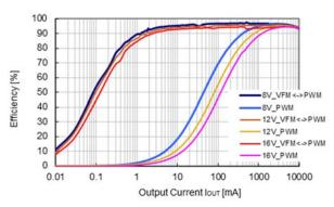
$V_{IN}$  = 12 V,  $V_{OUT}$  = 3.3 V  $f_{OSC}$ =500 kHz, MODE=L VFM/PWM auto-switching
