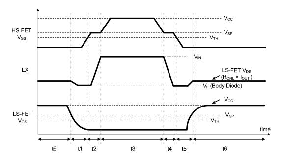
DCDC Converter Basic Switching Timing Chart
