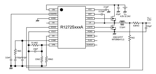
R1272SxxxA Typical Application Circuit at 500 kHz
