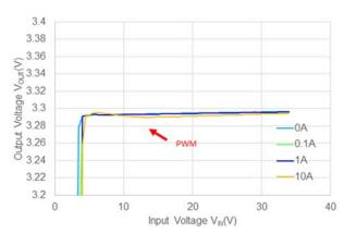
14) Up-down tracking  $V_{IN} = 12 \text{ V}, V_{OUT} = 3.3 \text{ V}$   $f_{OSC} = 500 \text{ kHz}, \text{MODE} = \text{H}$  Forced PWM
