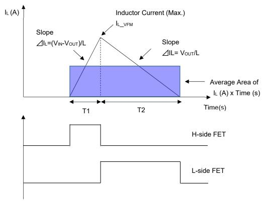
**Inductor Current Waveform at VFM Mode**
