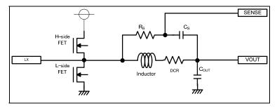
Figure B Detecting with Inductor's DCR
