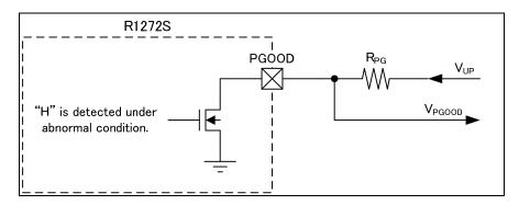
**PGOOD Output Pin Connecting Diagram**
