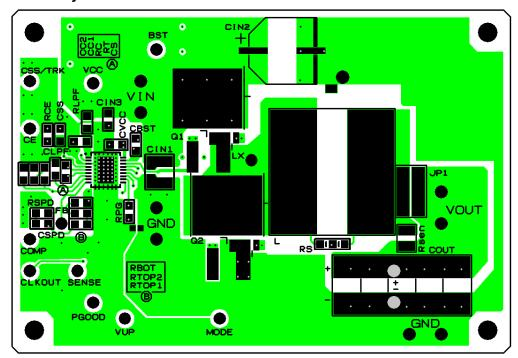
PCB Layout – 1<sup>st</sup> Layer (Top Layer)
