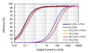
$V_{OUT} = 5.0 \text{ V}$  $f_{OSC} = 250 \text{ kHz} / V_{IN} = 8 \text{ V} / 12 \text{ V} / 16 \text{ V}$
