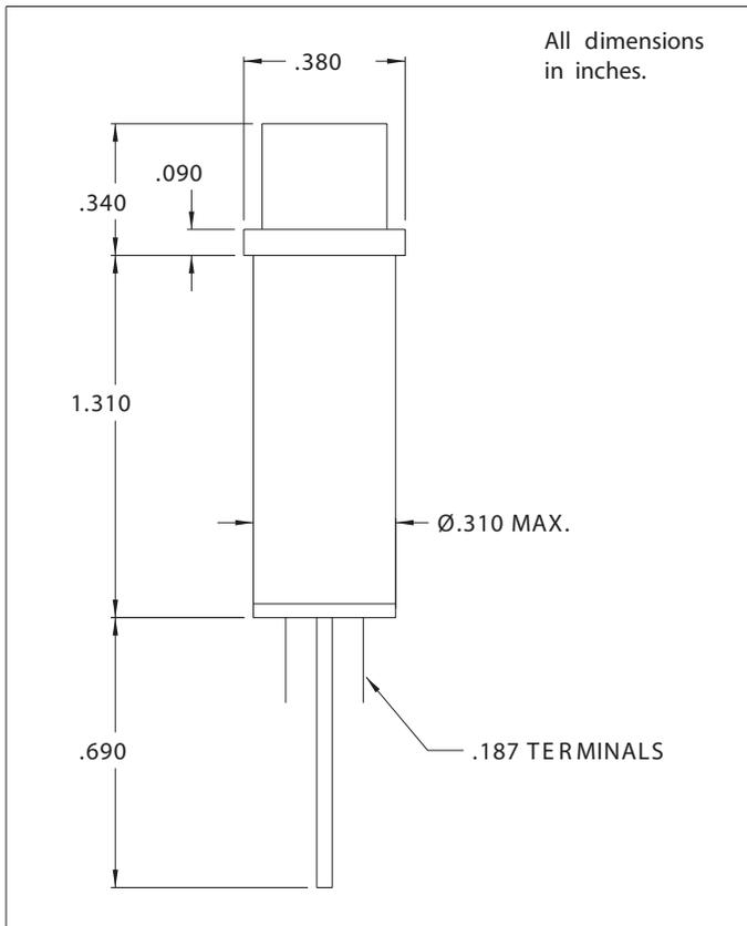
Mounting: Ø.310 MIN., supplied with push-on speednut SN1287.
