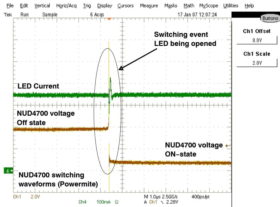
Figure 8. NUD4700 Switching Waveforms
