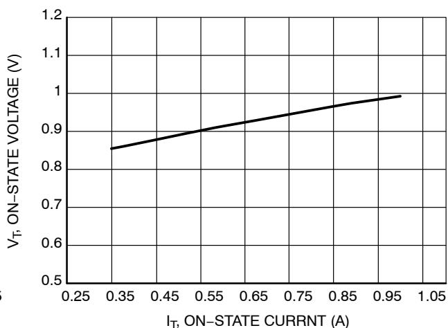
Figure 6. On-State Voltage vs. On-State Current (I<sub>T</sub>) at 25°C
