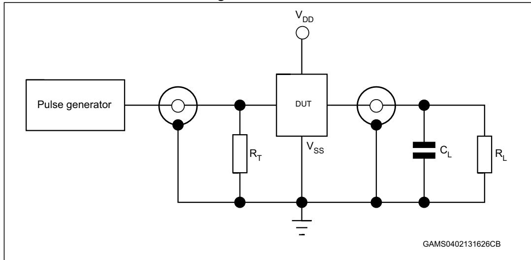
1. Legend:  $C_L = 50 \text{ pF}$  or equivalent (includes jig and probe capacitance),  $R_L = 200 \text{ K}\Omega$ ,  $R_T = Z_{OUT}$  of pulse generator (typically 50  $\Omega$ )
