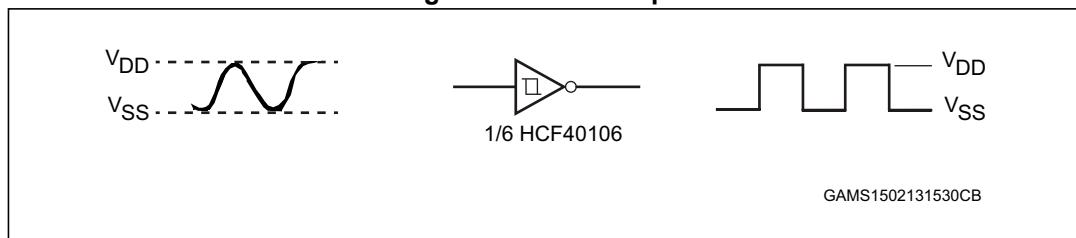
The frequency range of the wave shape is from DC to 1 MHz.
