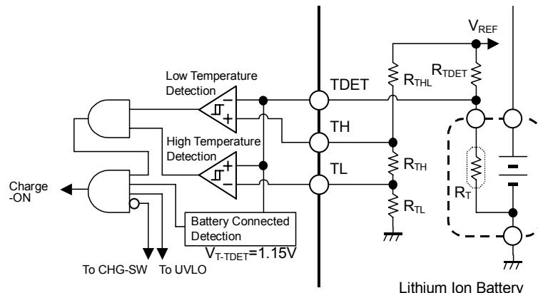
Figure 4 Temperature Detection Block
