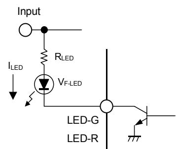
Figure 5. LED Drive Circuit
