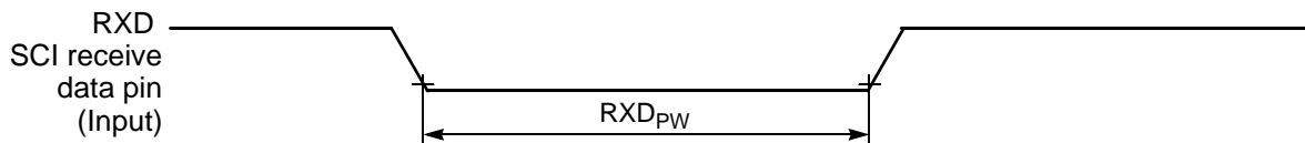
Figure 10-17 RXD Pulse Width
