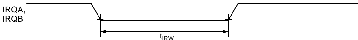
Figure 10-7 External Interrupt Timing (Negative Edge-Sensitive)
