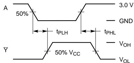
**Figure 4. Switching Waveforms**
