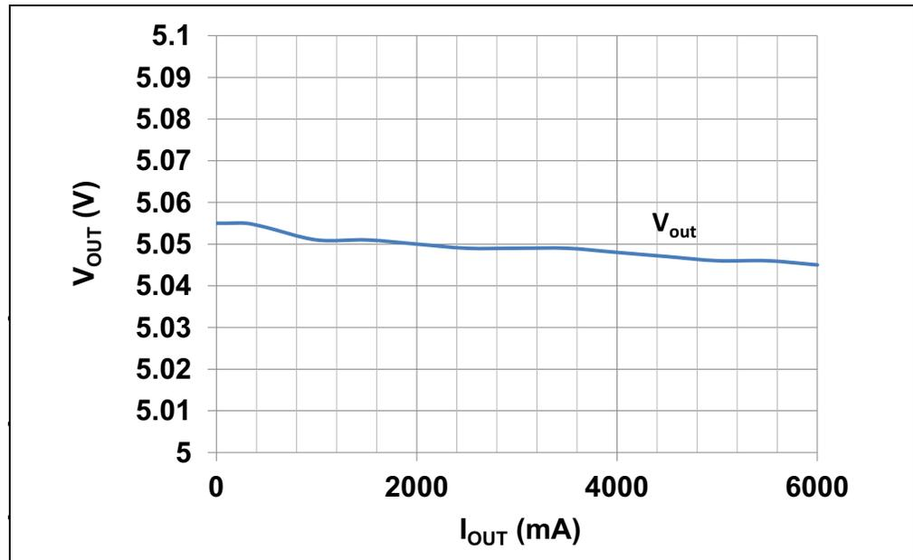
**FIGURE C-2:** Load Regulation ( $V_{IN} = 24V$ ).
