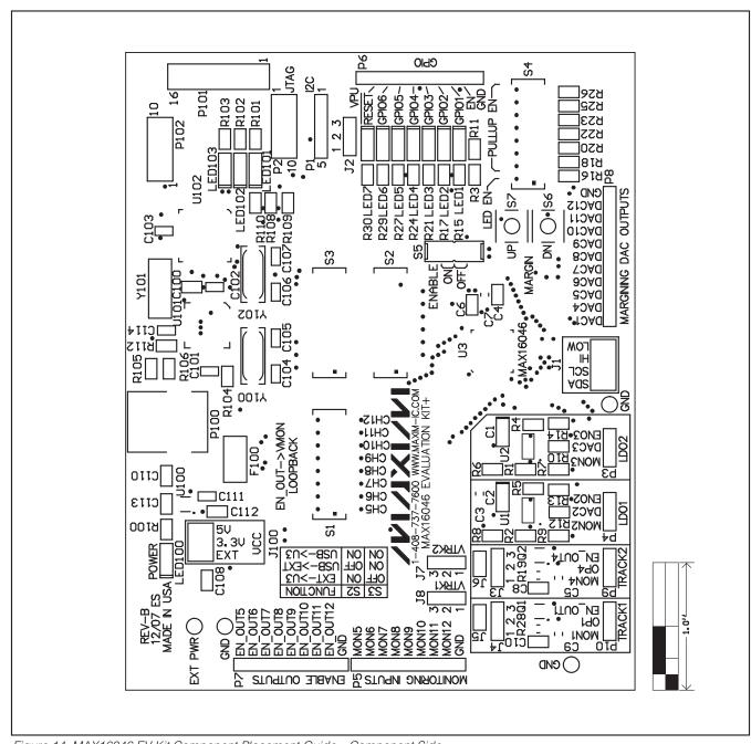
Figure 14. MAX16046 EV Kit Component Placement Guide—Component Side
