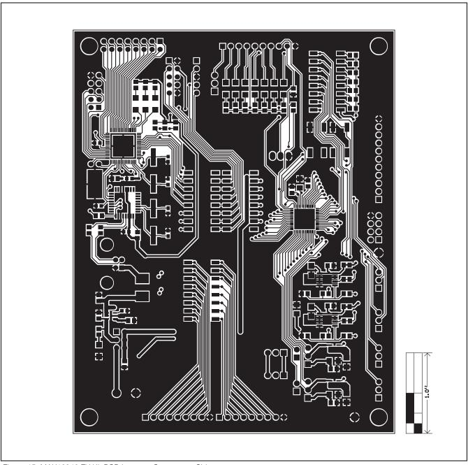
Figure 15. MAX16046 EV Kit PCB Layout—Component Side
