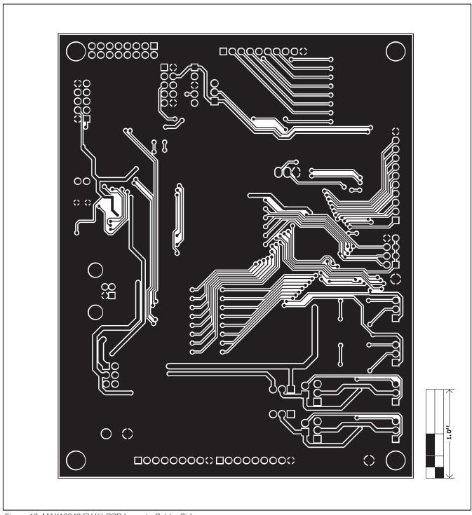
Figure 16. MAX16046 EV Kit PCB Layout—Solder Side
