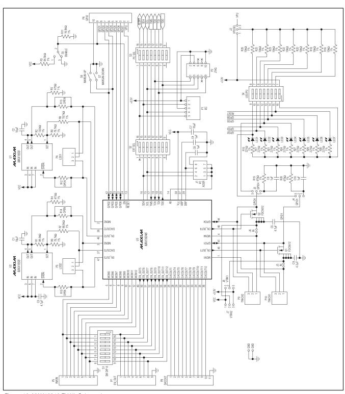
Figure 12. MAX16046 EV Kit Schematic
