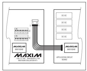
Figure 9. Connecting the EV Kit to an External Application Board Using  $\rm I^2C$
