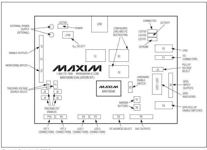
Figure 11. Evaluation Kit PCB Diagram
