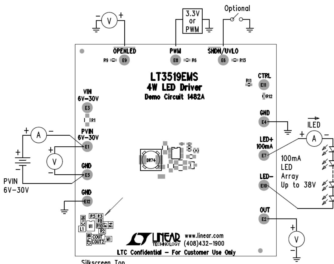
Figure 3. Proper Measurement Equipment Setup
