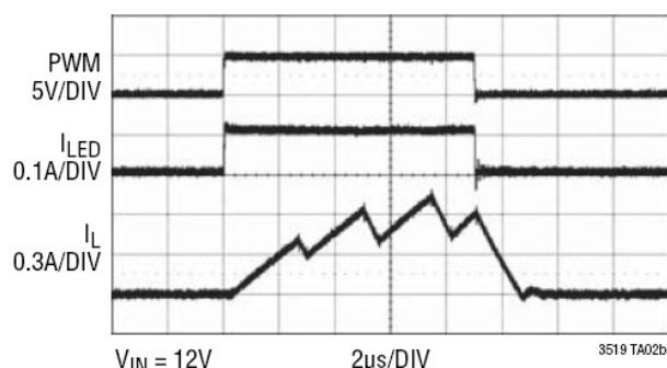
Figure 2. DC1482A 38V LED string PWM Dim, VIN=12V
