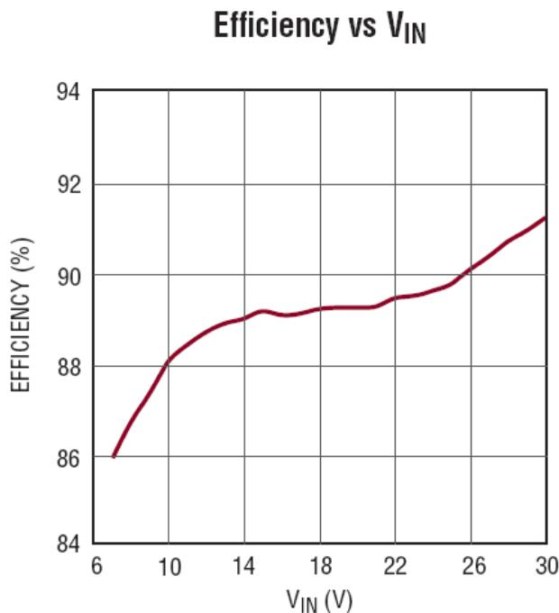
Figure 1. DC1482 Efficiency vs. VIN 38VLED at 100mA
