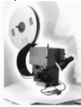
[Semi-automatic crimping machine, [Contact withdrawal tool] applicator]
