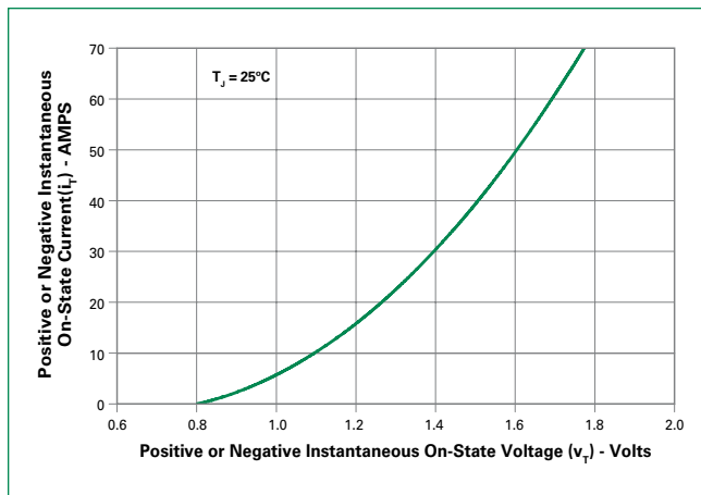
Figure 9: On-State Current vs. On-State Voltage (Typical)
