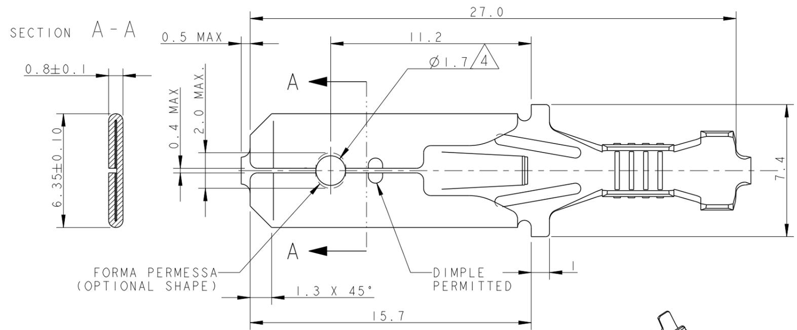
1) STATO DI FORNITURA (SUPPLY CONDITION, Scala 1:1)
