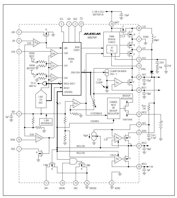
Figure 1. MAX769 Block Diagram
