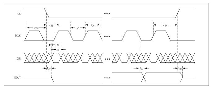
Figure 4. Detailed Serial-Interface Timing
