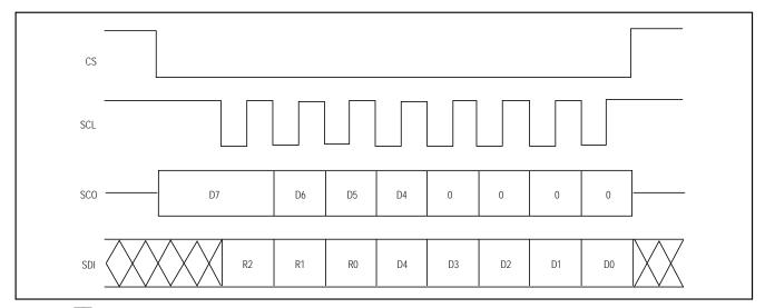
Figure 5. CS, SCL, SDO, and SDI Serial Timing
