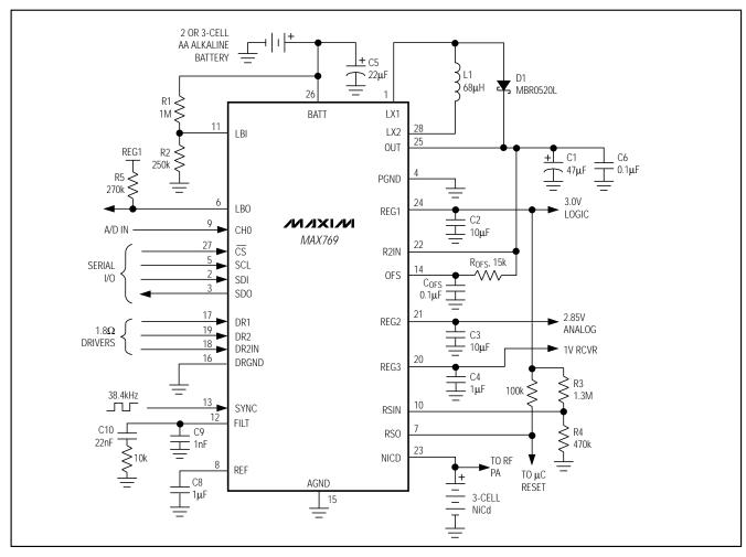
Figure 2. Standard Application Circuit
