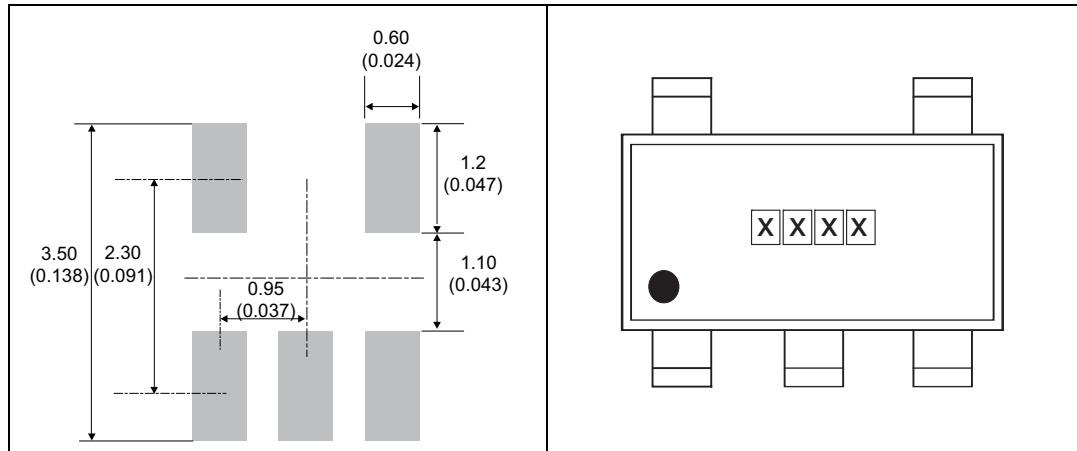
**Figure 8. Marking layout**
