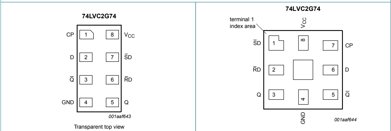
Fig. 5. Pin configuration SOT833-1, SOT1089, SOT1116 and SOT1203 (XSON8)
