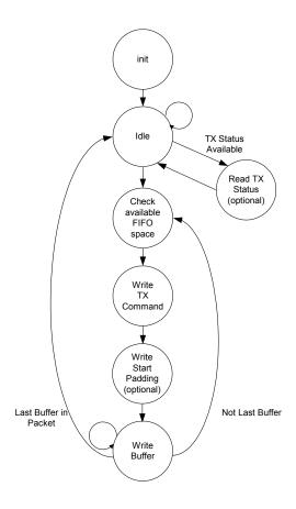
Figure 3.12 Simplified Host TX Flow Diagram
