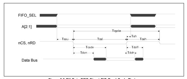
Figure 6.3 RX Data FIFO Direct PIO Read Cycle Timing
