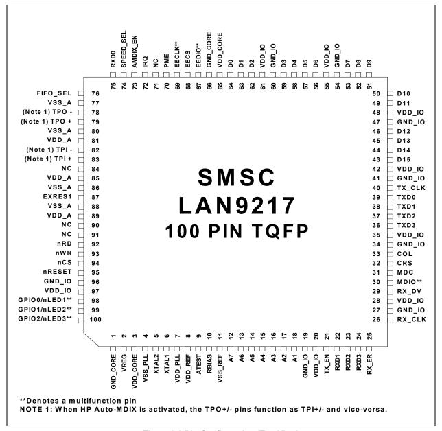
Figure 2.1 Pin Configuration (Top View)
