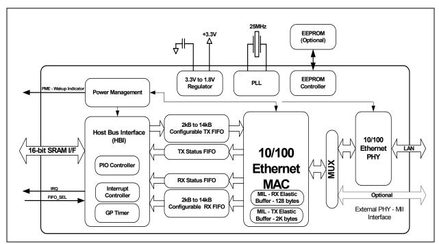
Figure 1.2 Internal Block Diagram
