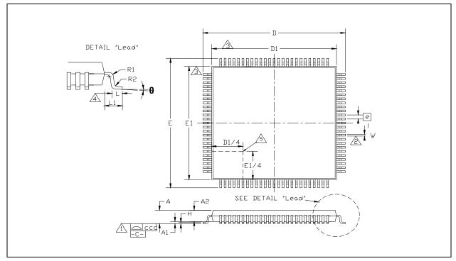
Figure 8.1 100 Pin TQFP Package Definition
