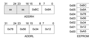
Figure 5.2 Example ADDRL, ADDRH and EEPROM Setup
