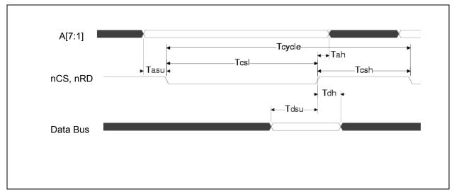
Figure 6.5 PIO Write Cycle Timing
