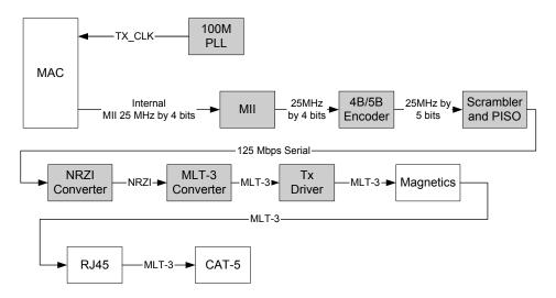
Figure 4.1 100Base-TX Data Path
