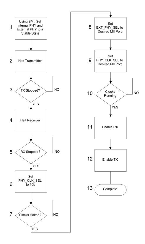
Figure 3.11 MII Switching Procedure
