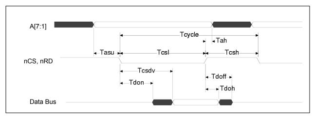
Figure 6.1 PIO Read Cycle Timing
