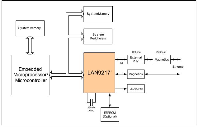
Figure 1.1 System Block Diagram
