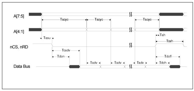
Figure 6.2 PIO Burst Read Cycle Timing
