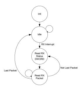
Figure 3.16 Host Receive Routine Using Interrupts
