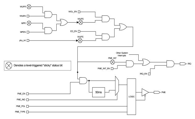
Figure 3.10 PME and PME\_INT Signal Generation
