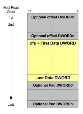
Figure 3.18 RX Packet Format
