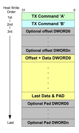
Figure 3.13 TX Buffer Format
