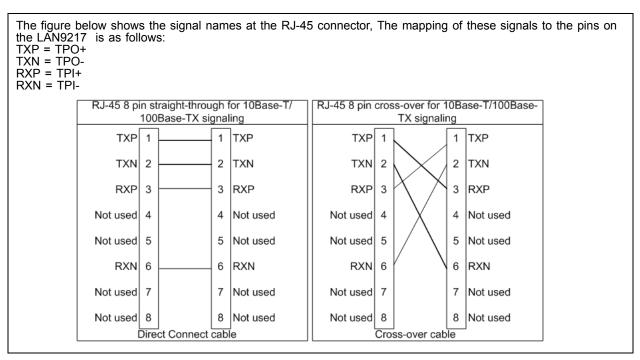
Figure 4.3 Direct cable connection vs. Cross-over cable connection.
