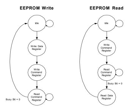
Figure 3.2 EEPROM Access Flow Diagram
