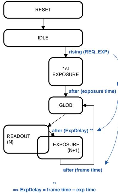
Because of the nature of the streaming mode, there is no such thing as invalid or special control timing. Once started, it will be forever looping and all further REQ\_EXP and REQ\_FRAME pulses are ignored.
