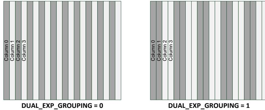
When **DUAL\_EXPOSURE** is set low, the exposure time of all pixels is set with **EXP\_TIME\_L**. When the register is set high, the exposure time of the two groups can be set independently with **EXP\_TIME\_S** and **EXP\_TIME\_L**.
