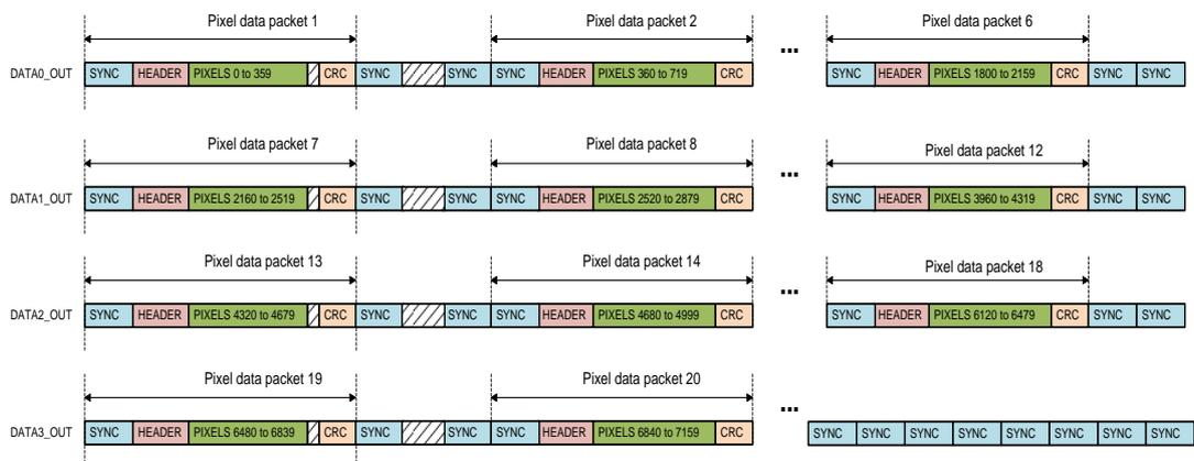
Every used data output channel outputs 6 data packets per line, separated by a number of empty packets.
