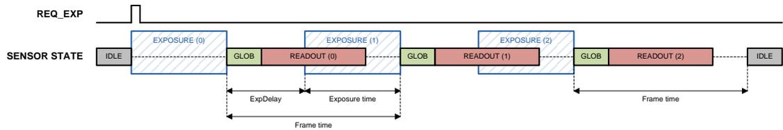
In the example, the programmed 'frame time' is longer than the sum of GLOB length and READOUT length. This situation is allowed and provides an easy mechanism to fine-tune frame rate.
