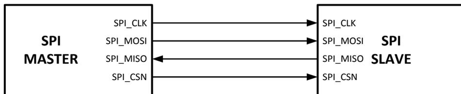
When using multiple CMV image sensors, the SPI\_CLK and SPI\_MOSI can be shared among them. The SPI\_CSN operates as a chip select for each of the slaves. The SPI\_MISO can also be shared on a bus because it is tri-stated when it is not used. This configuration of one master and multiple slaves is shown in Figure 22.
