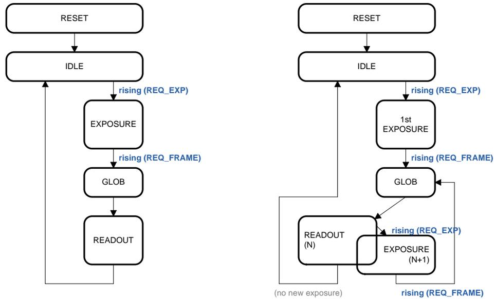
The length of the GLOB state, as well as the length of the READOUT period depends on a number of register settings.
