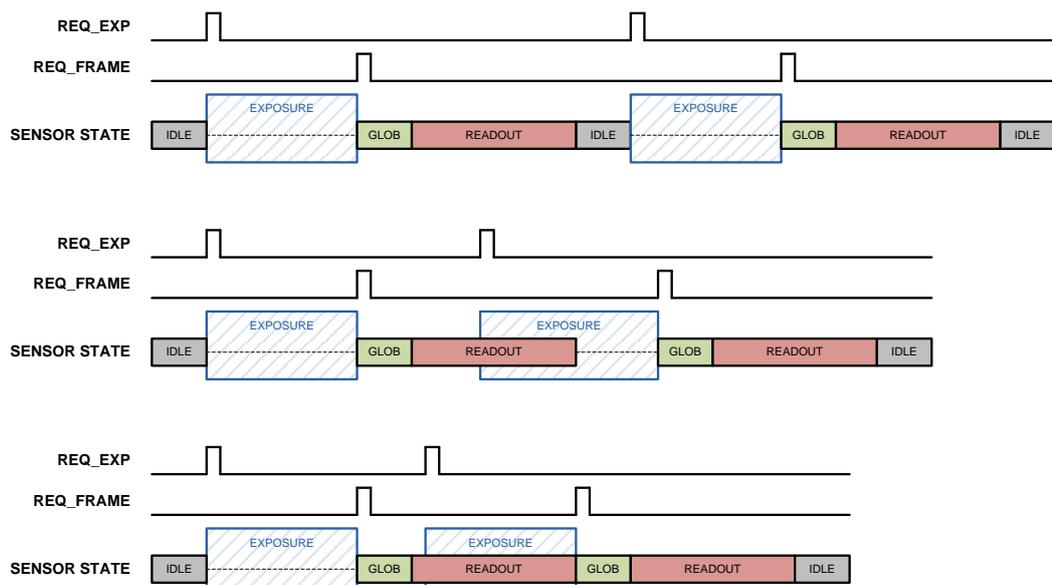
The figure shows how the *Full External* control mode can be used to (from top to bottom):
