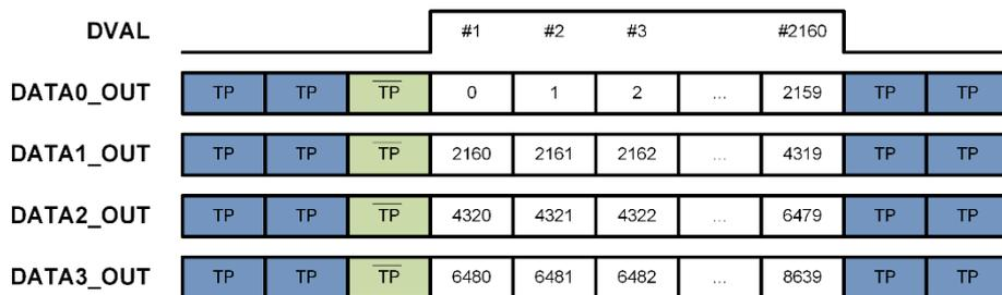
A similar example for packet-based readout format is given in Figure 113.
