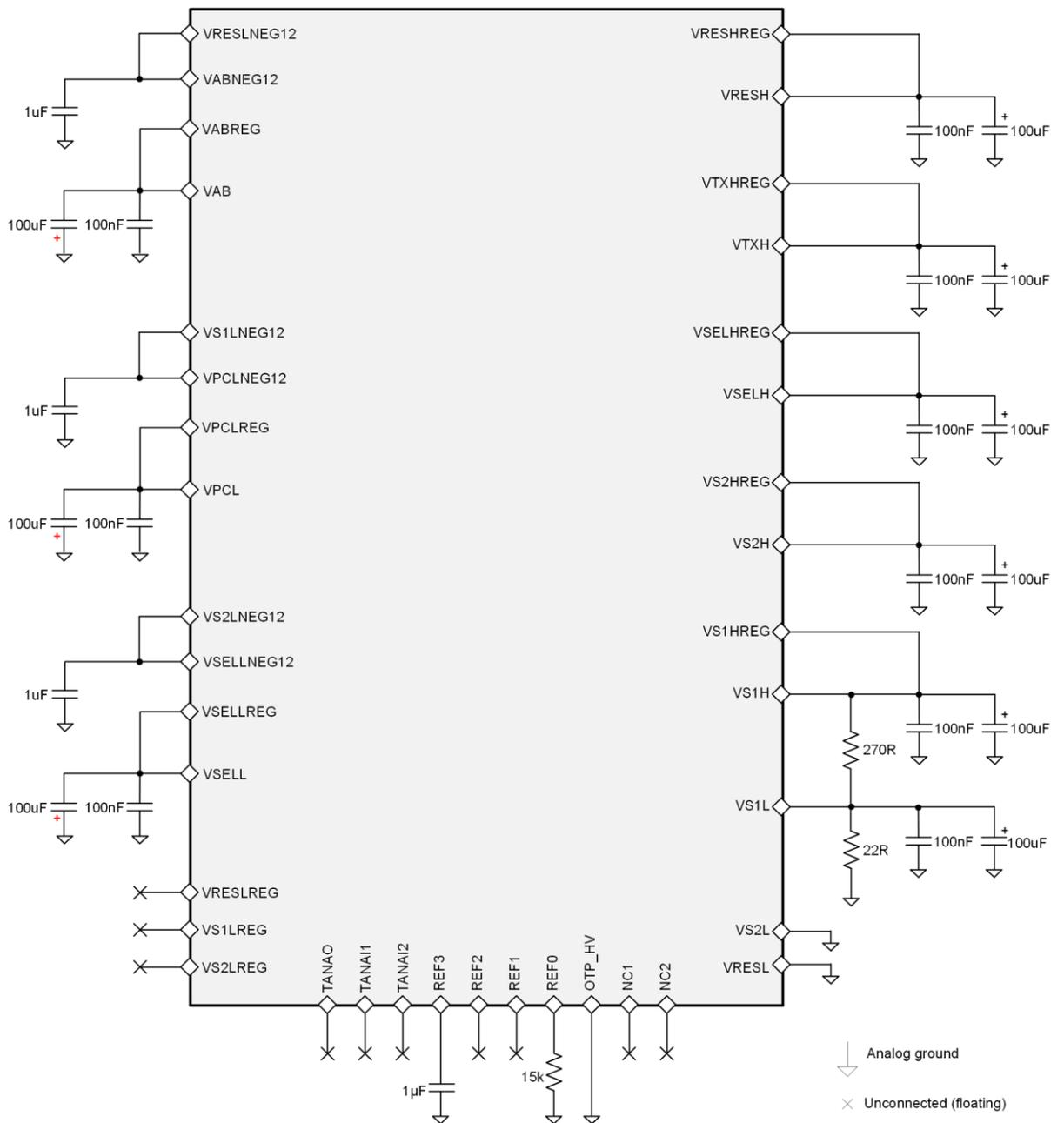
For the 100nF and 1µF capacitors, ceramic types can be used. Capacitances of 100µF can be electrolytic types (beware of the polarity on the negative supplies!). The maximal specified ESR and ESL of these 100µF capacitors are 0.1Ω and 10nH respectively.
