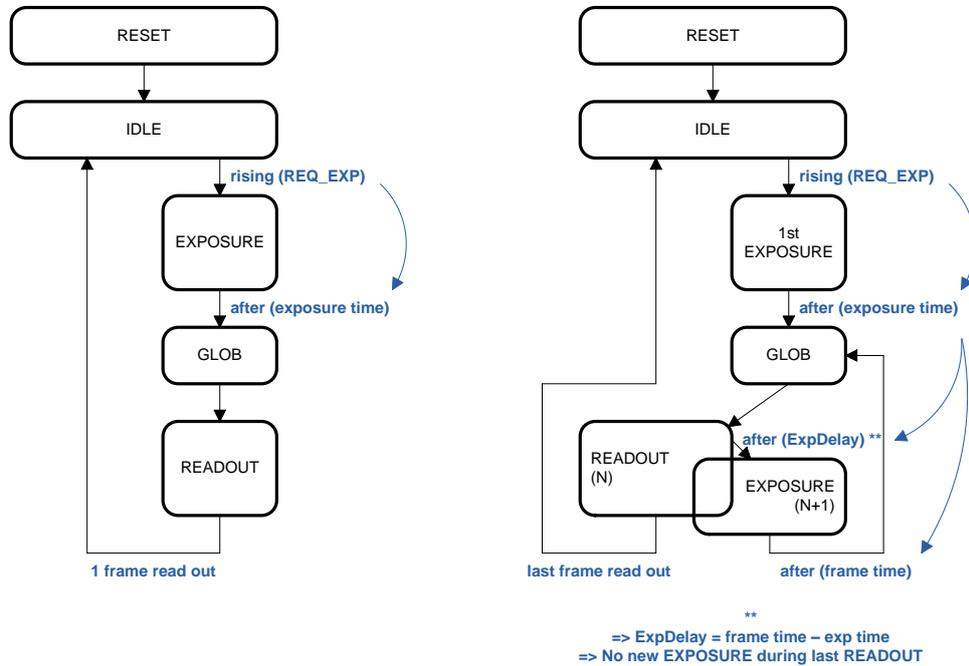
When exiting IDLE mode, the behavior is identical to Programmed External mode: a rising edge on REQ\_EXP will initiate the EXPOSURE state, which ends after a register defined exposure time. When the exposure time expires, a GLOB state is started, followed by READOUT.
