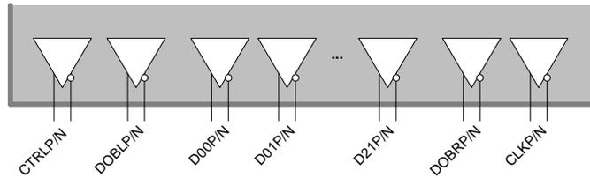
Each pair of differential output pins transports data on one sub-LVDS channel.
