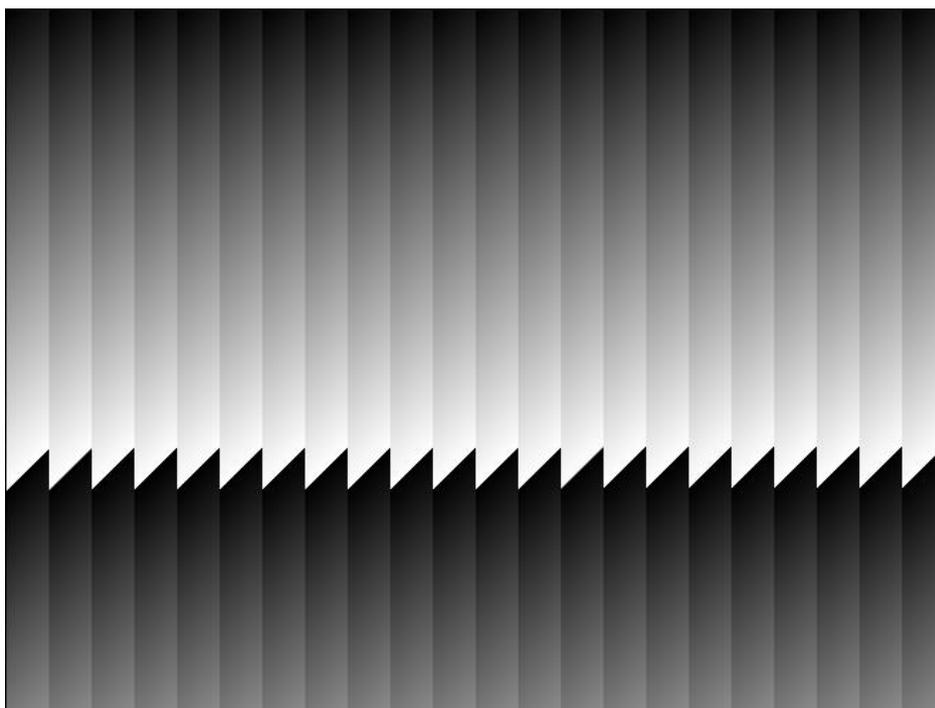
In sub-LVDS test mode 3, the actual data of every pixel is replaced by the output of a pseudo-random generator. The value of the first valid pixel of a frame is 4095. All outputs drive the same output value (unlike test mode 2, where the  $N_{\text{KERNEL}}$  generates an offset between outputs).
