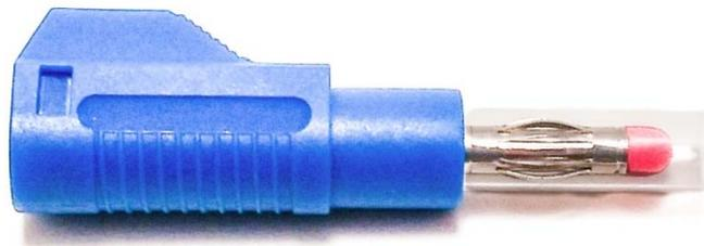
The BU-3261410 has a spring loaded retractable sheath that provides electrical protection when the cable is not mounted and slides into the housing when pressed into a non-shrouded jack. It also has a built-in banana jack that allows stacking other test leads with retractable or unshrouded 4mm banana plugs.
