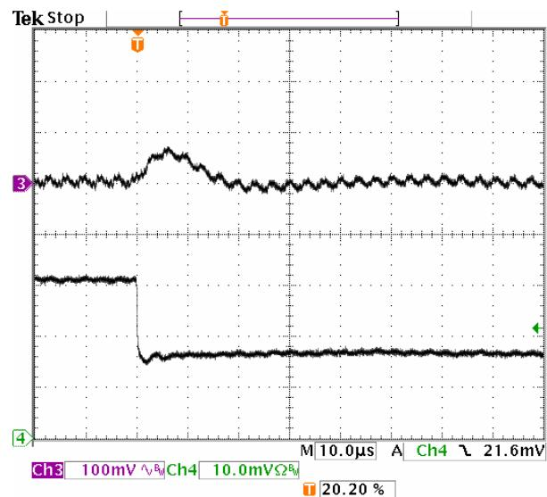
**Fig-1.5V-7:** Output voltage response for  $V_{out}=1.5V$  to positive load current step-change from 3A to 1.5A with slew rate of  $-5A/\mu s$  at  $V_{in}=5.0V$ .  $C_o=47\mu Fx2$  ceramic.
