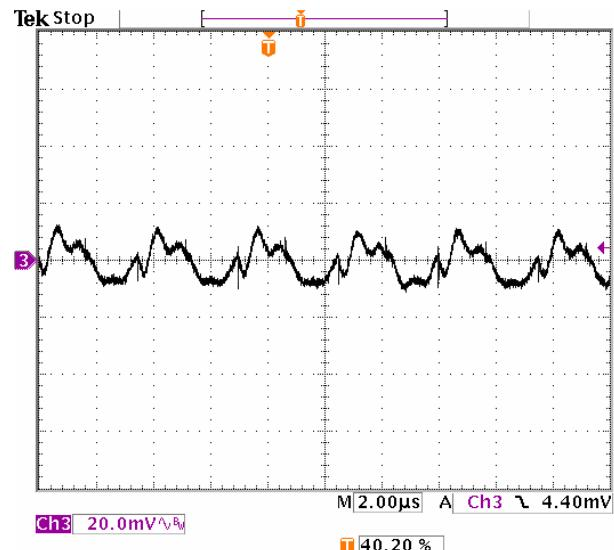
**Fig-2.5V-5:** Output voltage ripple (20mV/div.) for  $V_{out}=2.5V$  at full rated load current into a resistive load with external capacitance  $47\mu Fx2$  ceramic +  $1\mu F$  ceramic at  $V_{in}=5.0V$ . Time scale: 2μs/div
