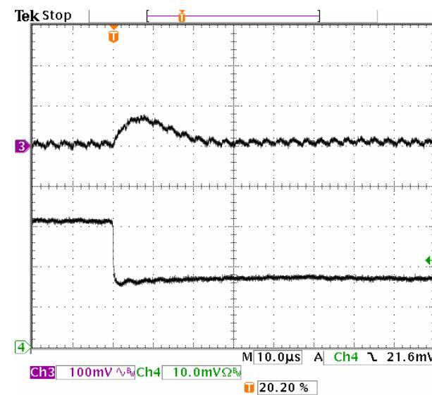
**Fig-1.0V-7:** Output voltage response for  $V_{out}=1.0V$  to positive load current step-change from 3A to 1.5A with slew rate of  $-5A/\mu s$  at  $V_{in}=5.0V$ .  $C_o=47\mu Fx2$  ceramic.
