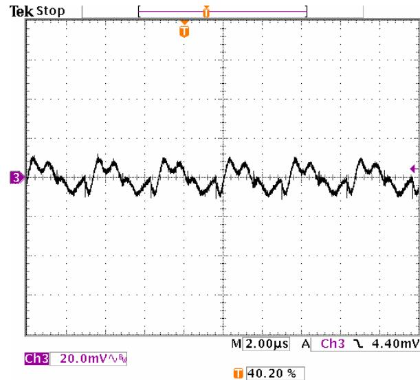
**Fig-2.0V-5:** Output voltage ripple (20mV/div.) for  $V_{out}=2.0V$  at full rated load current into a resistive load with external capacitance  $47\mu Fx2$  ceramic +  $1\mu F$  ceramic at  $V_{in}=5.0V$ .
