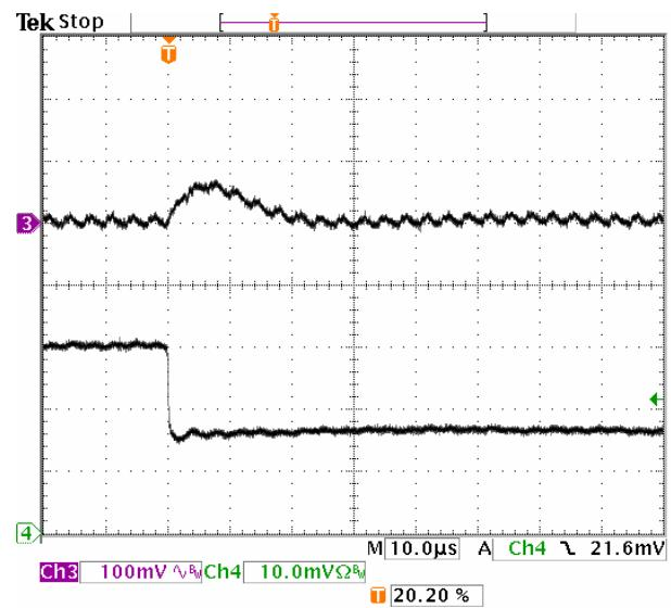
**Fig-0.7525V-7:** Output voltage response for  $V_{out}=0.7525V$  to positive load current step-change from  $3A$  to  $1.5A$  with slew rate of  $-5A/\mu s$  at  $V_{in}=5.0V$ .  $C_o=47\mu Fx2$  ceramic.
