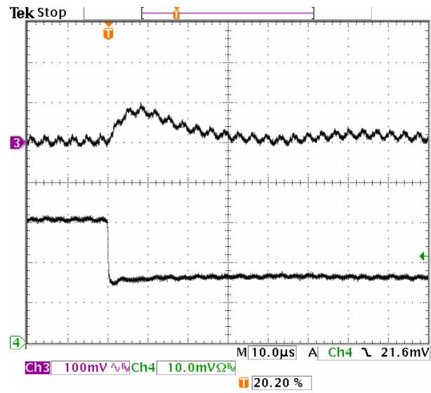
**Fig-2.5V-7:** Output voltage response for  $V_{out}=2.5V$  to positive load current step-change from  $3A$  to  $1.5A$  with slew rate of  $-5A/\mu s$  at  $V_{in}=5.0V$ .  $C_o=47\mu Fx2$  ceramic.
