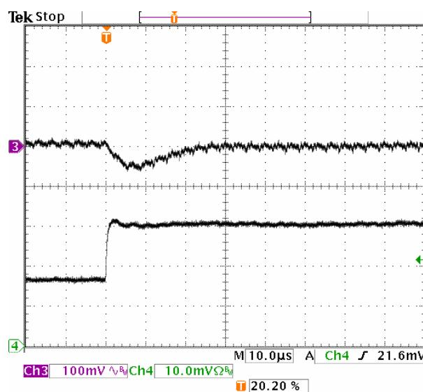
**Fig-1.0V-6:** Output voltage response for  $V_{out}=1.0V$  to positive load current step-change from 1.5A to 3A with slew rate of  $5A/\mu s$  at  $V_{in}=5.0V$ .  $C_o=47\mu Fx2$  ceramic.
