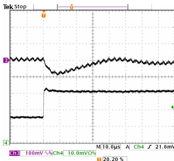
**Fig-3.3V-6:** Output voltage response for  $V_{out}=3.3V$  to positive load current step-change from 1.5A to 3A with slew rate of  $5A/\mu s$  at  $Vin=5.0V$ .  $Co=47\mu Fx2$  ceramic.
