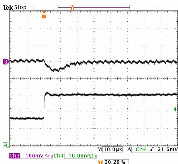
**Fig-0.7525V-6:** Output voltage response for  $V_{out}=0.7525V$  to positive load current step-change from  $1.5A$  to  $3A$  with slew rate of  $5A/\mu s$  at  $V_{in}=5.0V$ .  $C_o=47\mu Fx2$  ceramic.
