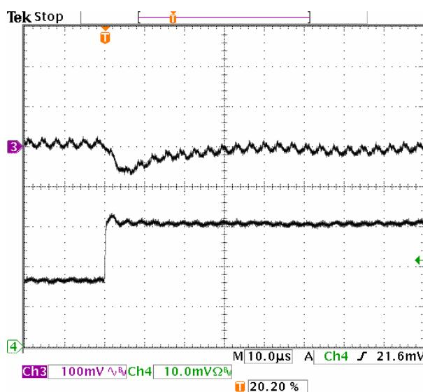
**Fig-2.5V-6:** Output voltage response for  $V_{out}=2.5V$  to positive load current step-change from  $1.5A$  to  $3A$  with slew rate of  $5A/\mu s$  at  $V_{in}=5.0V$ .  $C_o=47\mu Fx2$  ceramic.
