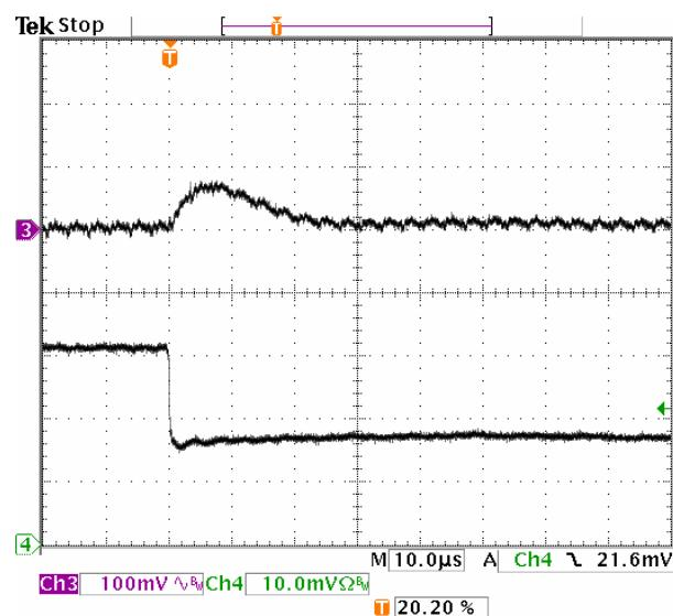
**Fig-1.2V-7:** Output voltage response for  $V_{out}=1.2V$  to positive load current step-change from 3A to 1.5A with slew rate of  $-5A/\mu s$  at  $V_{in}=5.0V$ .  $C_o=47\mu Fx2$  ceramic.
