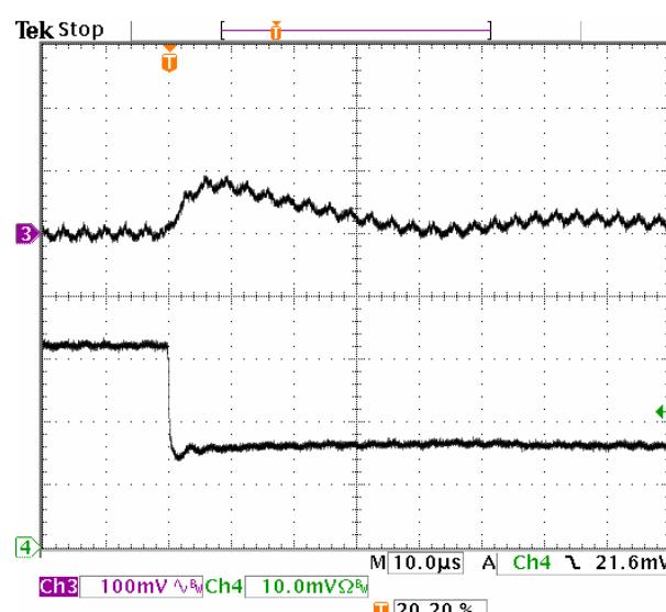
**Fig-3.3V-7:** Output voltage response for  $V_{out}=3.3V$  to negative load current step-change from 3A to 1.5A with slew rate of  $-5A/\mu s$  at  $Vin=5.0V$ .  $Co=47\mu Fx2$  ceramic.
