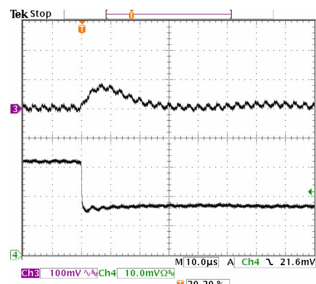
**Fig-2.0V-7:** Output voltage response for  $V_{out}=2.0V$  to positive load current step-change from 3A to 1.5A with slew rate of  $-5A/\mu s$  at  $V_{in}=5.0V$ .  $C_o=47\mu Fx2$  ceramic.
