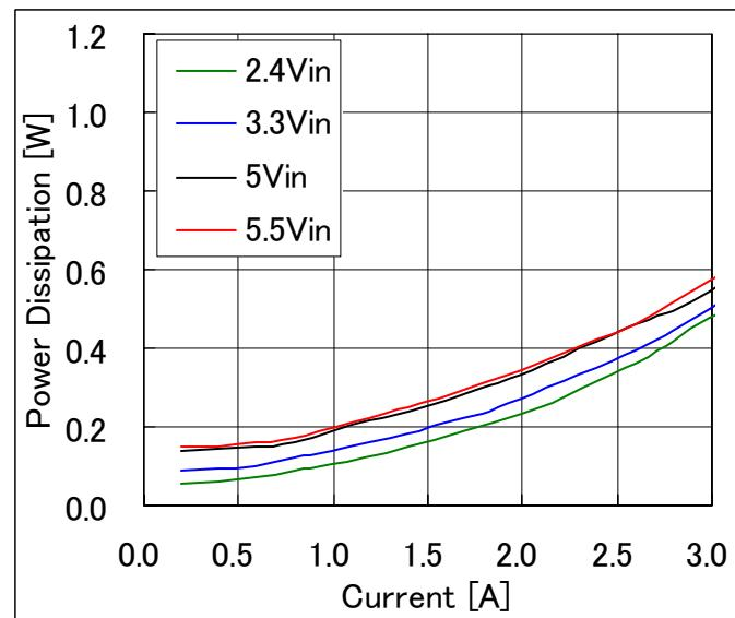
**Fig-1.2V-3:** Power dissipation vs. load current and input voltage for  $V_{out}=1.2V$ .
