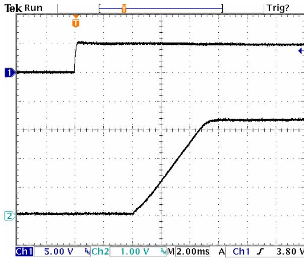
**Fig-3.3V-4:** Turn-on transient for  $V_{out}=3.3V$  with application of  $V_{in}$  at full rated load current (resistive) and  $47\mu Fx2$  external capacitance at  $Vin=5.0V$ .
