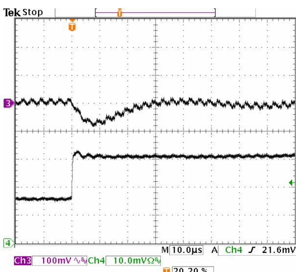
**Fig-2.0V-6:** Output voltage response for  $V_{out}=2.0V$  to positive load current step-change from 1.5A to 3A with slew rate of  $5A/\mu s$  at  $V_{in}=5.0V$ .  $C_o=47\mu Fx2$  ceramic.
