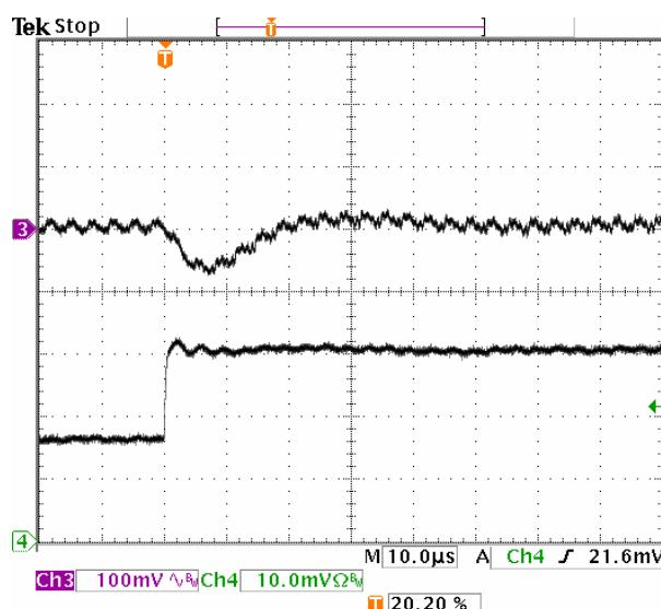
**Fig-1.5V-6:** Output voltage response for  $V_{out}=1.5V$  to positive load current step-change from 1.5A to 3A with slew rate of  $5A/\mu s$  at  $V_{in}=5.0V$ .  $C_o=47\mu Fx2$  ceramic.
