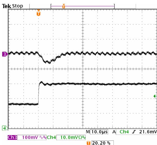
**Fig-1.2V-6:** Output voltage response for  $V_{out}=1.2V$  to positive load current step-change from 1.5A to 3A with slew rate of  $5A/\mu s$  at  $V_{in}=5.0V$ .  $C_o=47\mu Fx2$  ceramic.
