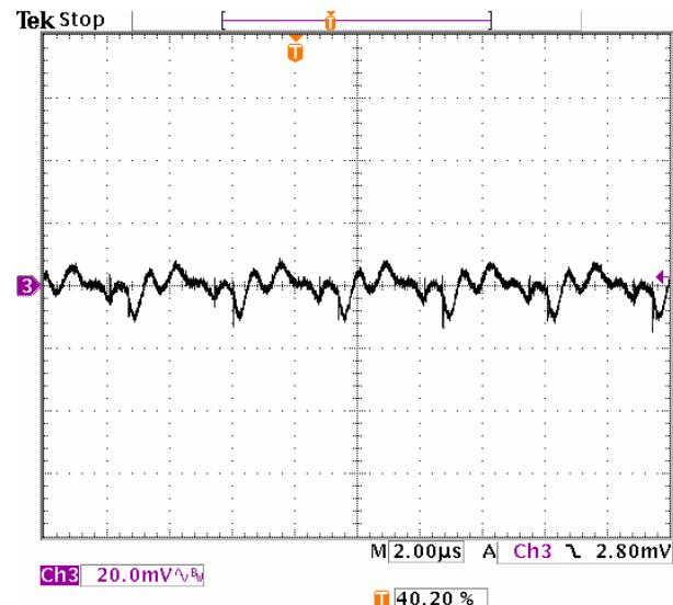
**Fig-0.7525V-5:** Output voltage ripple (20mV/div.) for  $V_{out}=0.7525V$  at full rated load current into a resistive load with external capacitance  $47\mu Fx2$  ceramic +  $1\mu F$  ceramic at  $V_{in}=5.0V$ .
