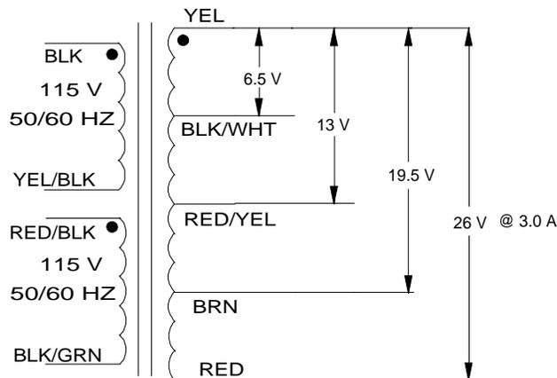
**Technical note:** Primary windings are designed to be connected in series or parallel.
