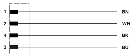
Contact assignment of the M8 plug
