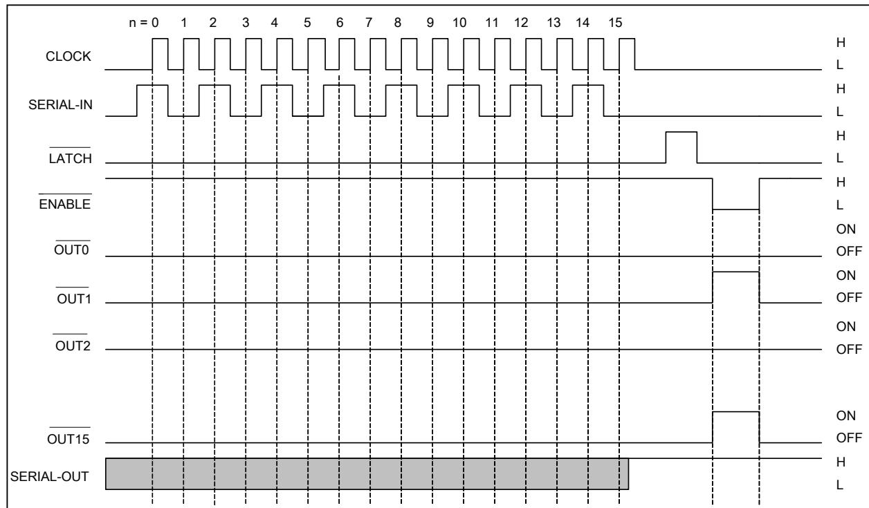
Figure 3 Timing Diagram
