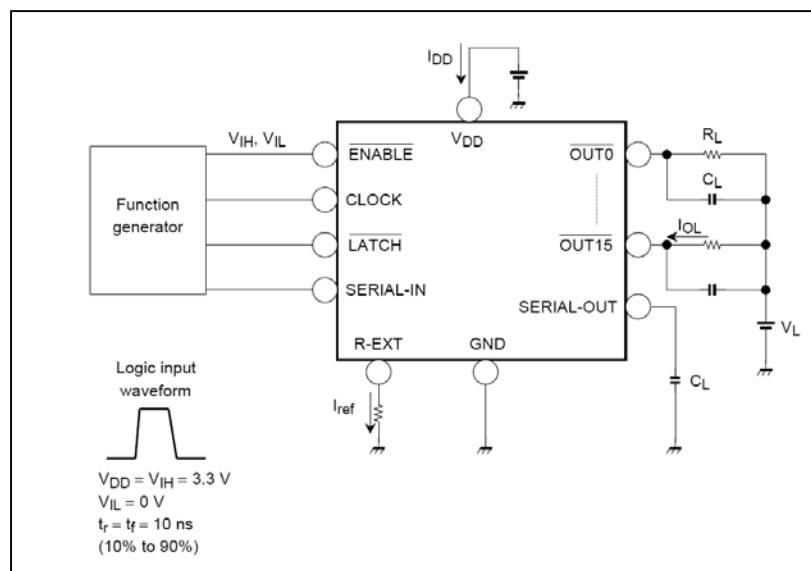
**Figure 4** Test Diagram
