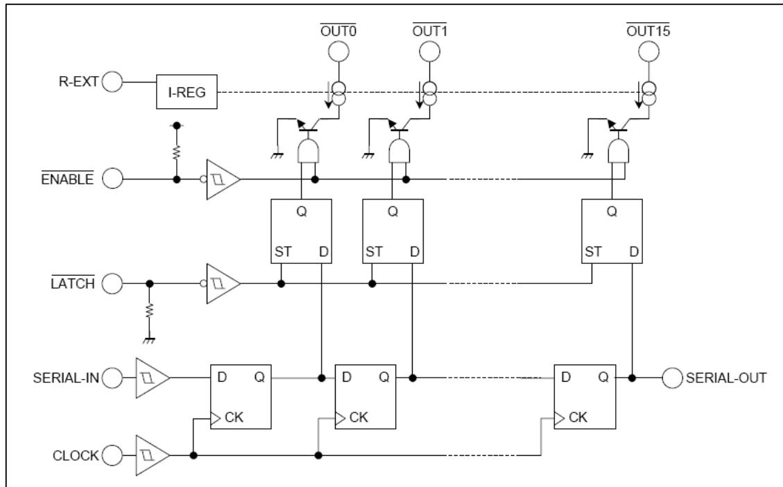
Figure 1 Block Diagram
