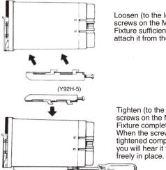
Loosen (to the left) the screws on the Mounting Fixture sufficiently and attach it from the bottom.
