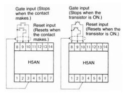
When connecting a solid-state circuit not of the open collector type to the gate or reset inputs as shown below, the voltage of the solid-state circuit (+V) should be 13 to 30 V, and the V<sub>CE(S)</sub> of the transistor should be less than 3 V (the current that flows from either terminal 9 or 10 is approximately 10 mA). Moreover, it is essential that the circuit be ON for gate or reset input, and OFF when there is no input.
