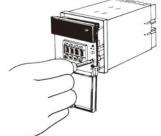
The internal unit comes out by loosening the internal unit fixing screw.
