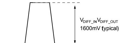
Figure 1b. Differential Voltage Swing
