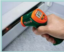
Test for temperature in heating systems
