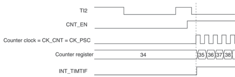
Figure 9-29. Control Circuit in Trigger Mode
