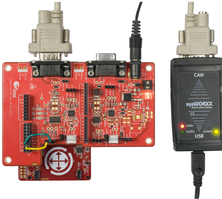
Figure 4-2. CAN Analyzer Connection to CY8CKIT-026's CAN1 Transceiver
