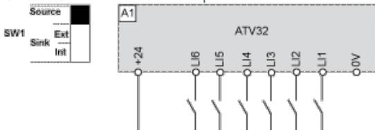
Switch SW1 set to "Source" position and use of an external power supply for the LIs
