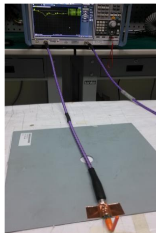
c) with 30*30cm Ground Metal Edge
