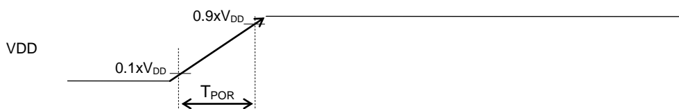
Power-on reset activation power rise time ( T_{POR} )
