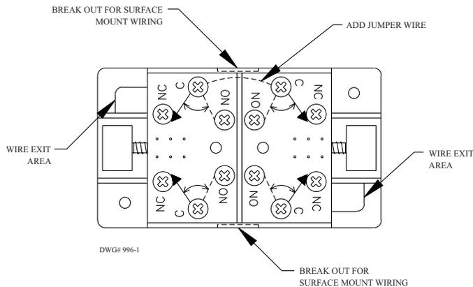
**Converting The HUB-T To Optional Latching Operation**
