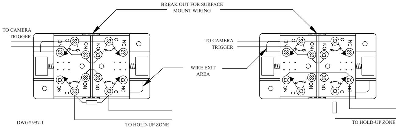
Electrical interlock requires both buttons to be activated simultaneously before alarm will occur. Any single button will activate camera.
